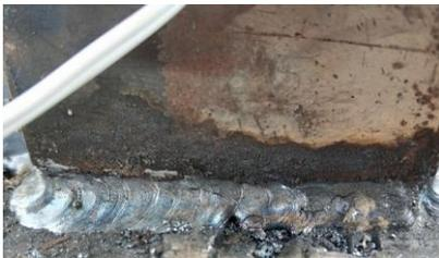
(d) Crack in welding seam at link to brace connection
