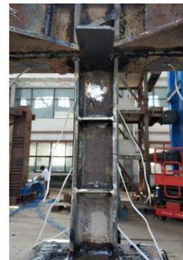
(c) Residual deformation of shear link
