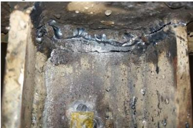
(g) Completely torn at link to beam connection
