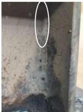
(a) Peeling of welding seam
