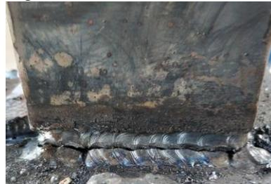
(h) Full fracture of welding seam at link flange to brace connection
