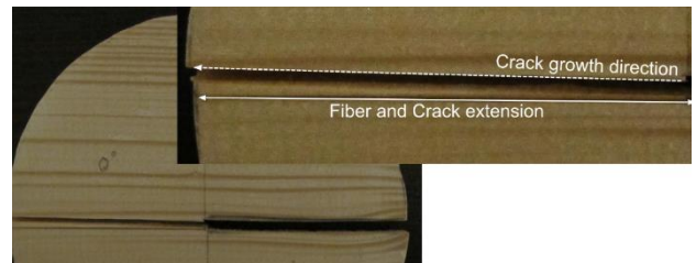
Fig. 6 The crack growth path in the matrix constrained between fibers
