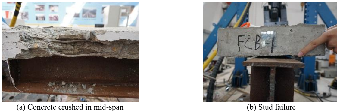
Fig. 4 Failure mode of test beams
