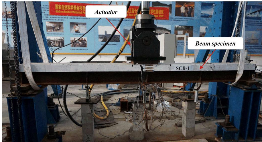
Fig. 2 The loading process of the test beam and the testing system
