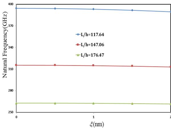
Fig. 8 Variation of fundamental natural frequencies of simply-supported nanoshell in terms of nonlocal parameter  $\xi$  for various dimensionless parameter of  $L/h$
