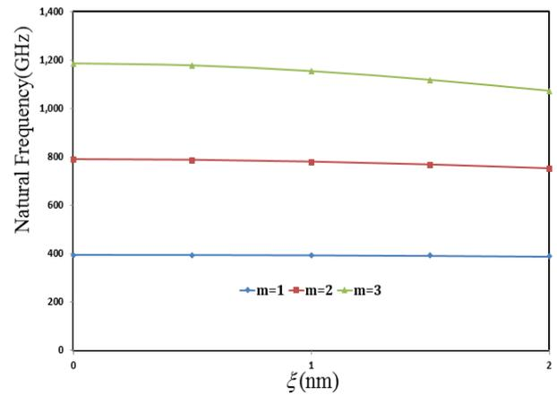
Fig. 6 The variation of natural frequencies of simply-supported functionally graded cylindrical nanoshell in terms of nonlocal parameter  $\xi$  for various modes  $m$
