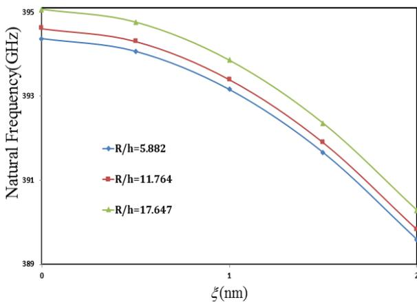
Fig. 9 Variation of fundamental natural frequencies of simply-supported nanoshell in terms of nonlocal parameter  $\xi$  for various dimensionless parameter of  $R/h$
