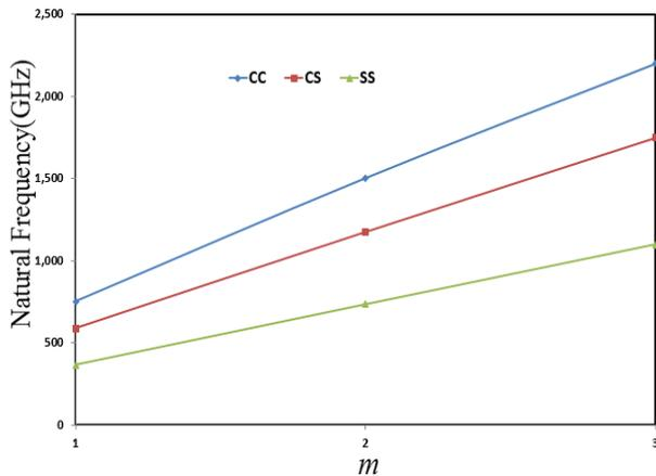
Fig. 12 Variation of fundamental natural frequencies of nanoshell in terms of mode number  $m$  for various boundary conditions
