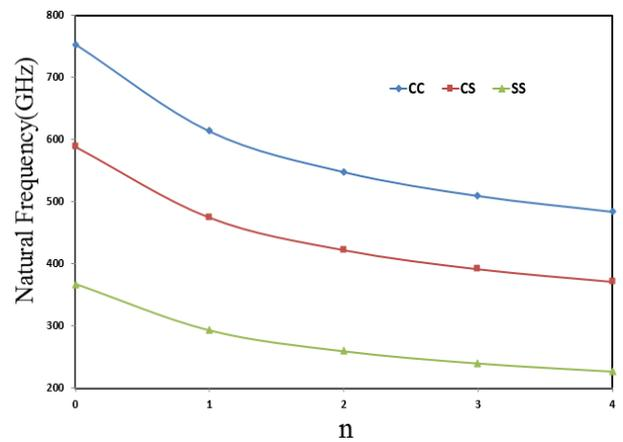
Fig. 11 Variation of fundamental natural frequencies of nanoshell in terms of in-homogeneous index  $n$  for various boundary conditions
