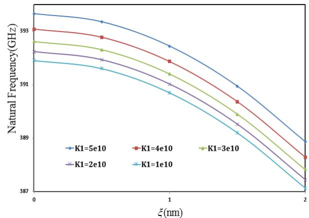
Fig. 3 The variation of fundamental natural frequencies of simply-supported functionally graded cylindrical nanoshell in terms of nonlocal parameters  $\xi$  for various Winkler's parameter  $K_1$
