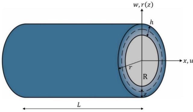
Fig. 1 The geometry and coordinate system of a cylindrical FGM nanoshell
