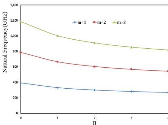
Fig. 5 The variation of natural frequencies of simply-supported functionally graded cylindrical nanoshell in terms of in-homogeneous index  $n$  for various modes  $m$
