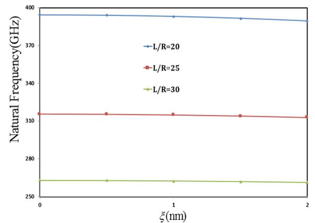
Fig. 7 Variation of fundamental natural frequencies of simply-supported nanoshell in terms of nonlocal parameter  $\xi$  for various dimensionless parameter of  $L/R$
