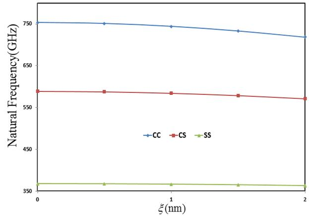
Fig. 10 Variation of fundamental natural frequencies of nanoshell in terms of nonlocal parameter  $\xi$  for various boundary conditions
