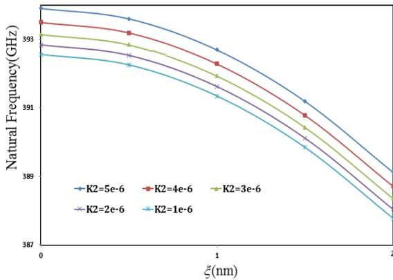
Fig. 4 The variation of fundamental natural frequencies of simply-supported functionally graded cylindrical nanoshell in terms of nonlocal parameters  $\xi$  for various Pasternak's parameter  $K_2$
