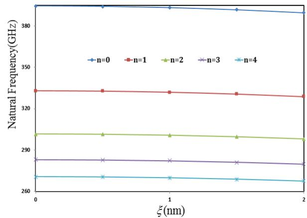
Fig. 2 The variation of fundamental natural frequencies of simply-supported functionally graded cylindrical nanoshell in terms of nonlocal parameters  $\xi$  for various in-homogeneous index  $n$
