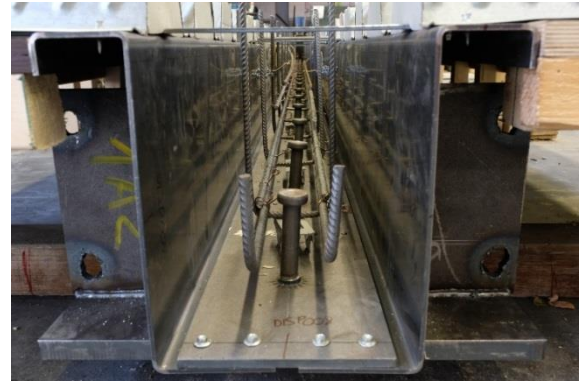
(b) U-shaped steel section and rebars
