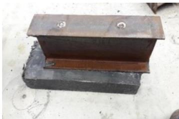
Fig. 10 Shear failure of welding material connecting stud to top flange
