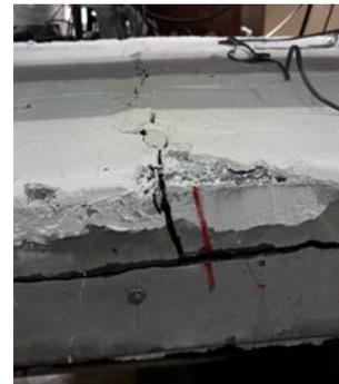
Fig. 14 Developed cracks in concrete slab over the interior support at ultimate load
