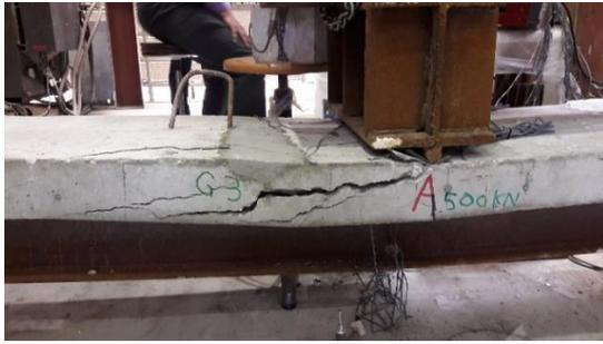
Fig. 16 Shear-compression failure at mid-span
