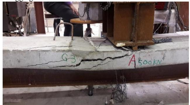
Fig. 26 Girder at failure stage
