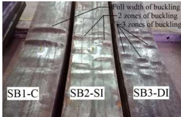
Fig. 4 Top flange local buckling failure for the tested CFST specimens
