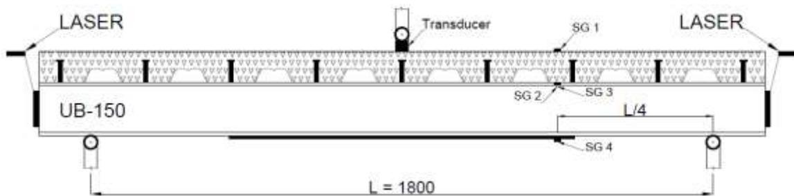
Fig. 8 Test set-up, location of transducer, strain gauges (SG) and LASER
