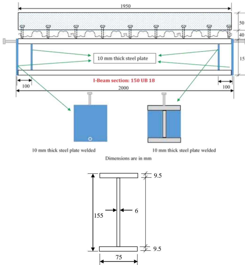
Fig. 2 Schematic of the control composite beam (not to scale)
