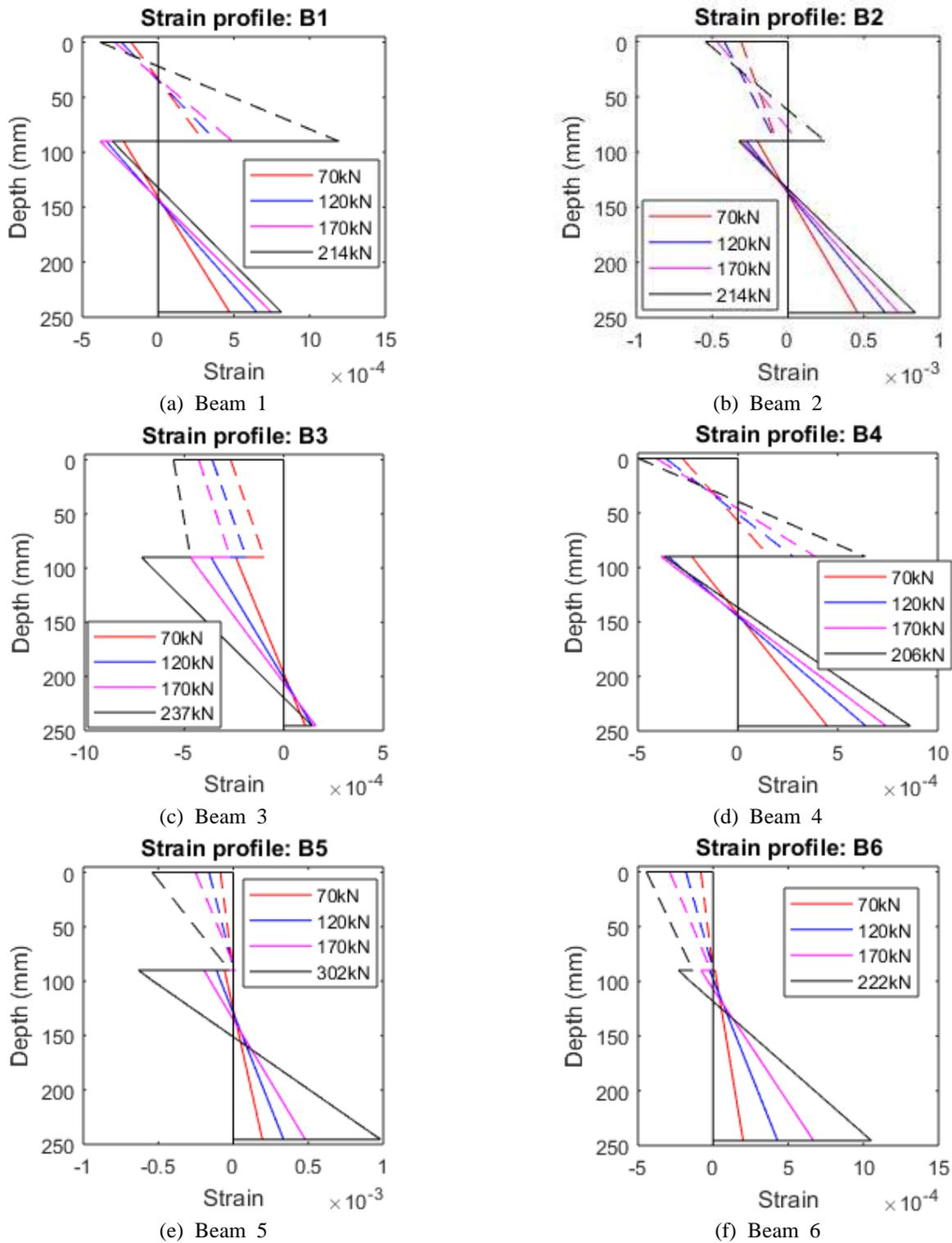
Fig. 13 Strain profile of all beams at different load level
