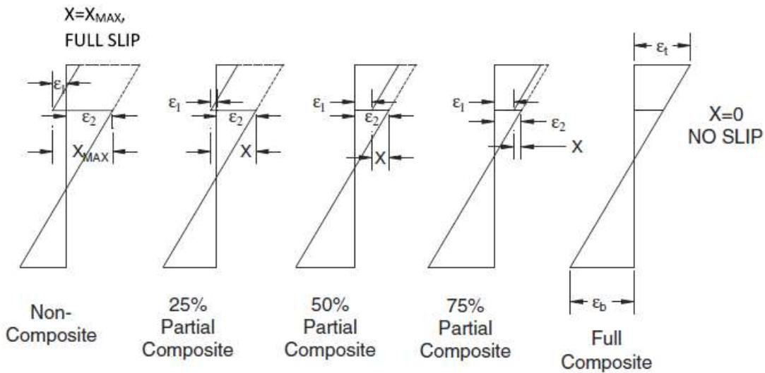
Fig. 14 Strain profile considering different degree of composite action (Chen and Yossef 2015)
