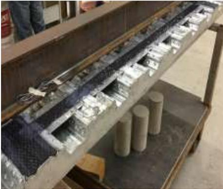
(a) attachment of CFRP on steel deck
