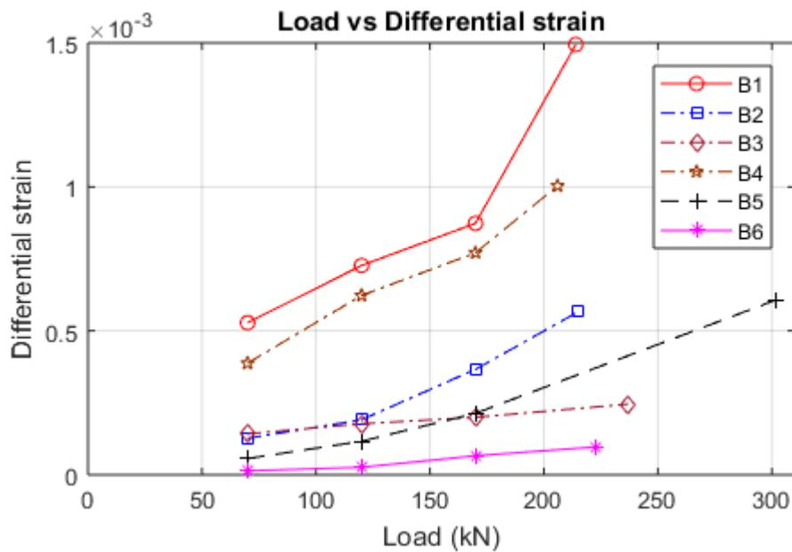
Fig. 15 Differential strain at various load level for all the beams
