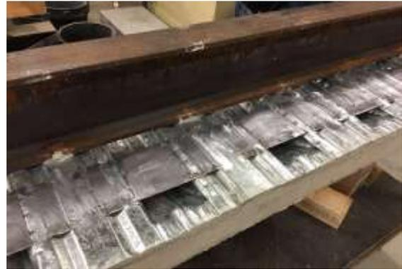
(b) steel plate welded on the deck to attach CFRP
