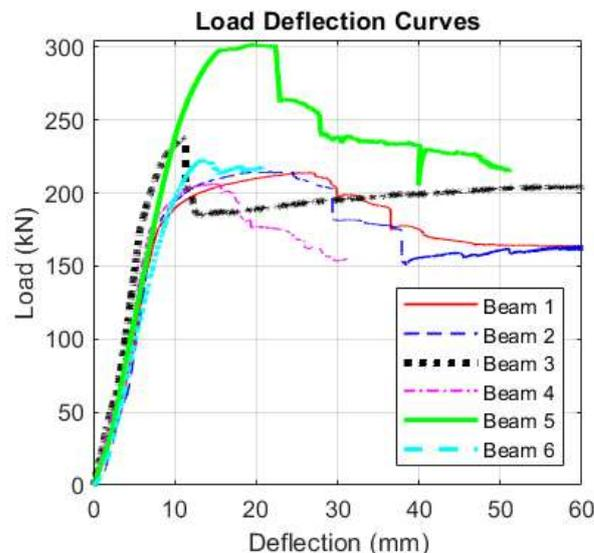
Fig. 9 Load-deflection curves of all the beams
