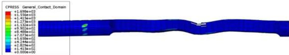
Fig. 21 Contact stress of TC50L20-A at average strain amplitude of 10%
