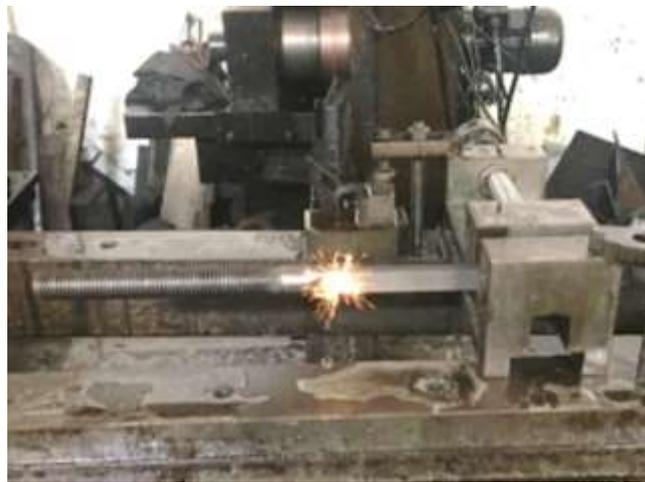
Fig. 4 Wire-electrode cutting process of specimens
