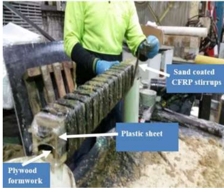
Fig. 4 The process of manufacturing the SCCFRP stirrups
