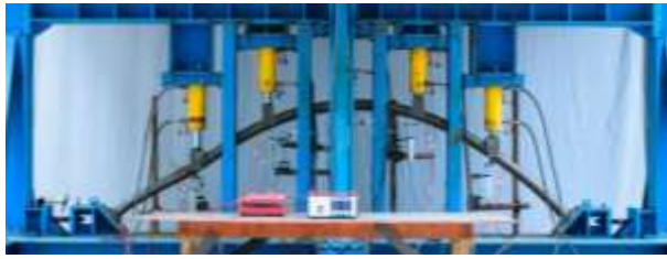
(a) Specimen 3 (asymmetric mode)
