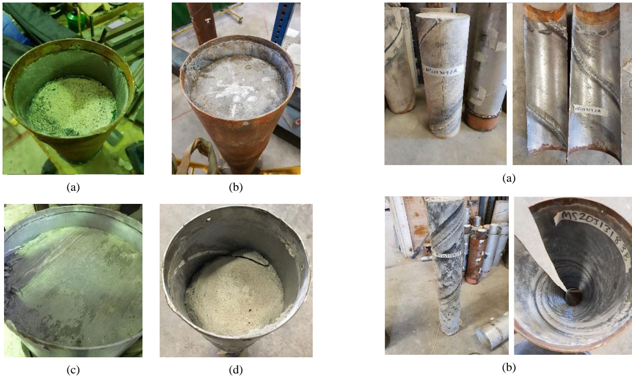
Fig. 4 Condition of the top end of the tested specimens at point of test termination (a) MSD1L12A; (b) MSD2L23; (c) SSD3L12B; d) SSD1L22A
