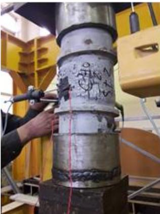
Fig. 8 Yielding Failure for specimen C40-2-St2
