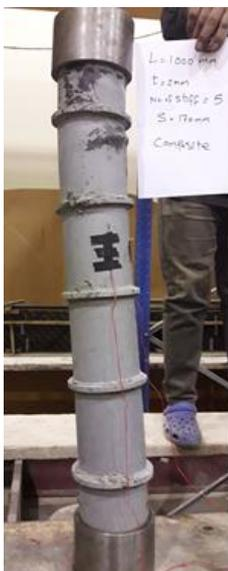
Fig. 9 Global Failure for specimen C100-2-St5
