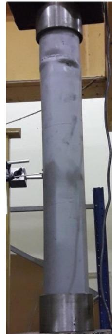
Fig. 6 Local Failure for specimen with steel only (short and medium columns)
