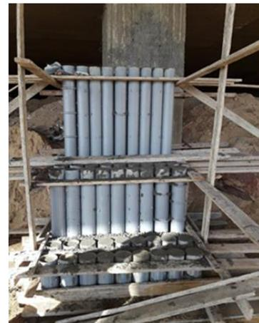
Fig. 3 Steel tubes after filling with concrete
