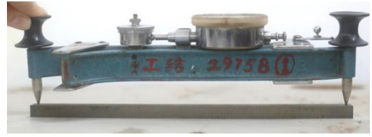
Fig. 8 Measurement of Whittemore strain gauge YB-25
