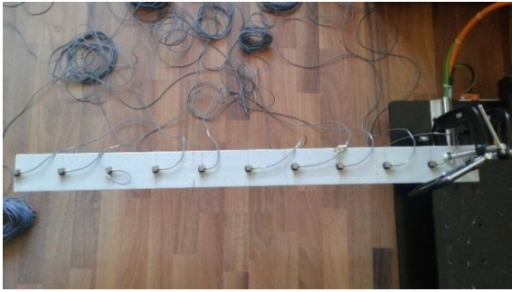
Fig. 3 The laboratory model of the cantilever composite beam for experimental measurements
