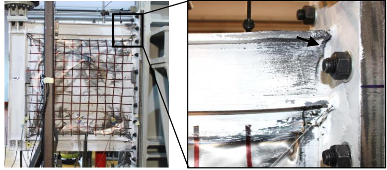
(c) At HAZ and propagation into column web at load step LS20b (specimen S60)
