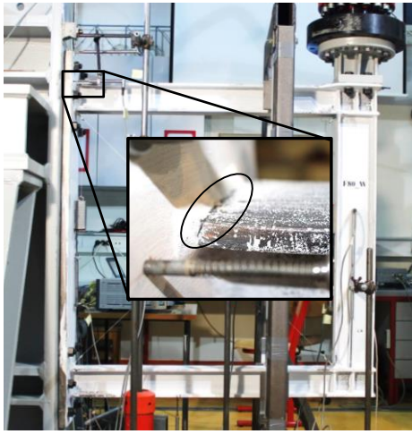
Fig. 11 Crack formation in HAZ at load step LS10 in specimen F80
