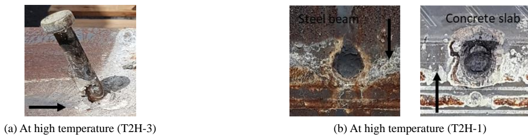
Fig. 10 Failure mode of the trapezoidal deck specimens with through-hole welding
