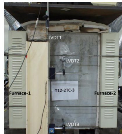
Fig. 3 Furnace and LVDT setup for the high-temperature experiment
