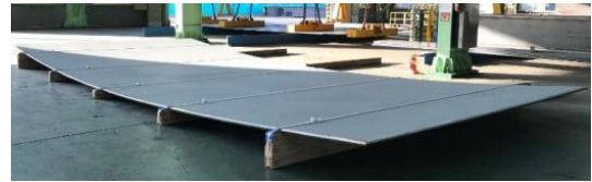
Fig. 7 Fabricated 25 mm, 4.5 m wide 9%Ni steel plate
