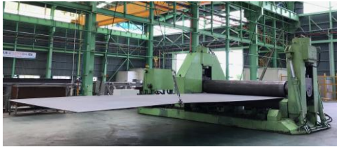
(b) Roll bending of 25 mm, 4.5 m wide plate
