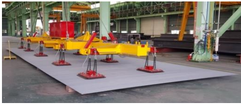
(a) 10 mm, 4.8 m wide plate handling with vacuum crane
