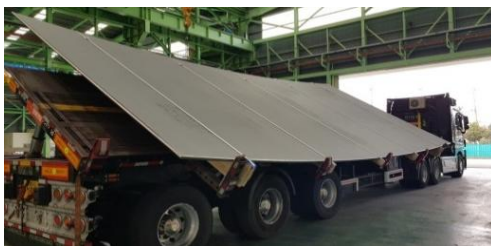
(c) 10 mm, 4.8 m wide plate sloping carriage
