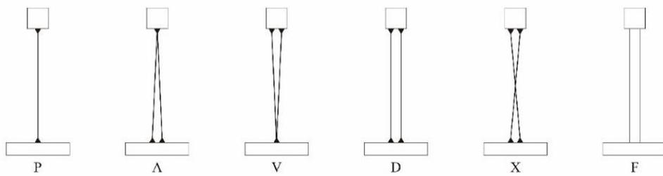
Fig. 30 Configurations of hangers within a plane perpendicular to the arch
