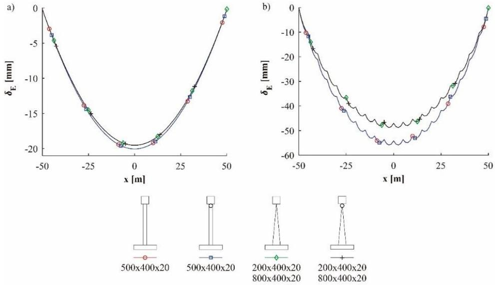
Fig. 28 Deflection at the edge of the deck under  $q_2$ : (a) Reference bridge; (b) Torsional stiffness of the deck factored by 0.2
