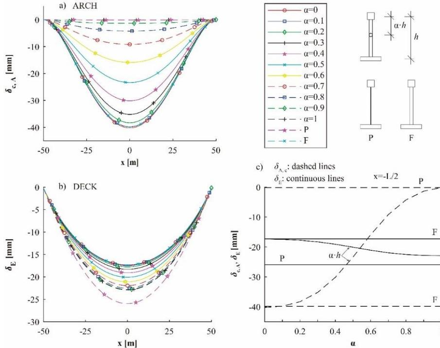
Fig. 21 (a) Transversal deflection at the crown under  $q_2$ ; (b) Vertical deflection at the edge of the deck under  $q_2$ ; (c) Detailed results at midspan
