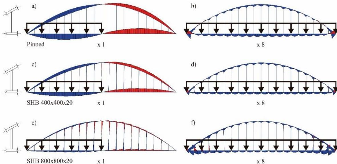
Fig. 15 Bending moment diagrams for the reference model (a, b), fixed SHB 400×400×20 mm stiffened hangers (c, d), and fixed SHB 800×800×20 mm stiffened hangers (e, f), for  $q_3$  (a, c, e) and the whole deck,  $q_5$  (b, d, f)
