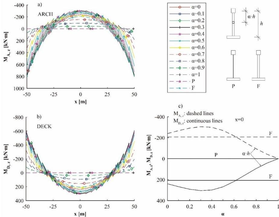
Fig. 19 Transversal arch (a) and deck (b) bending moment diagrams under  $q_2$  vs. hinge location; (c) Detailed results at midspan
