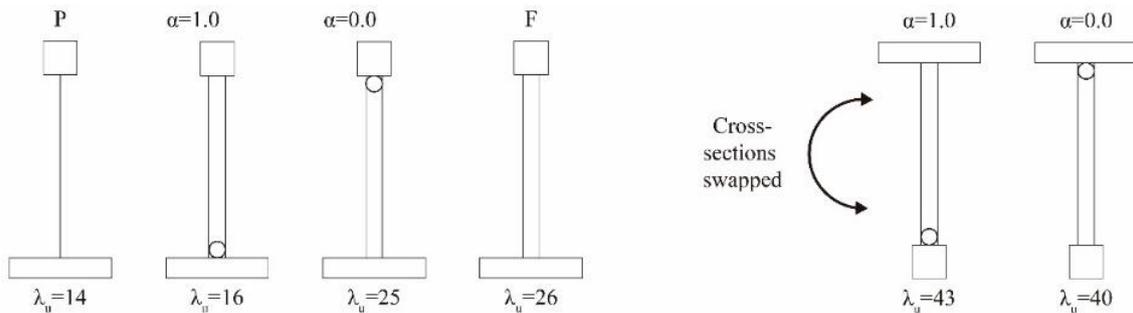
Fig. 26 Reference bridge: Coefficient  $\lambda_u$  for different hangers configuration, for load case  $B = 1.35 \cdot G + W + \lambda_u \cdot q_5$
