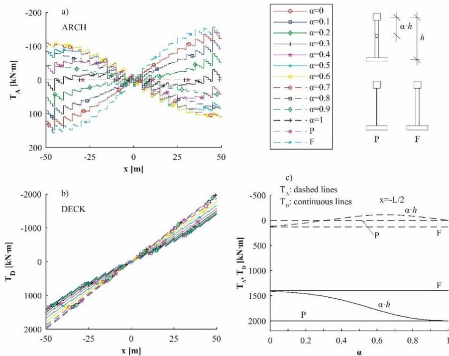
Fig. 20 Torsion under  $q_2$  at the arch (a) and the deck (b) vs. hinge location; (c) Detailed results at springings and abutments
