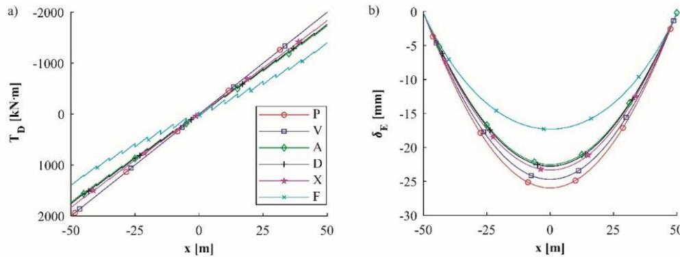
Fig. 32 Deck under  $q_2$ . (a) torsional moments; (b) deflections at the edge of the deck
