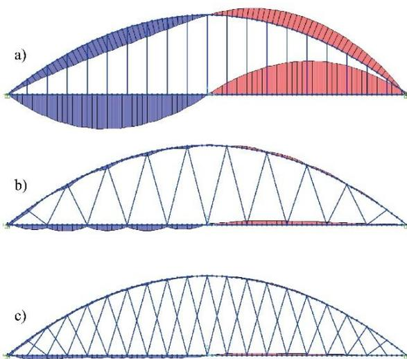
Fig. 4 Comparison of bending moment for different hanger arrangements, drawn at the same scale, under an UDL upon half the deck: (a) Vertical hangers; (b) Nielsen-Löhse hangers; (c) Network hangers
