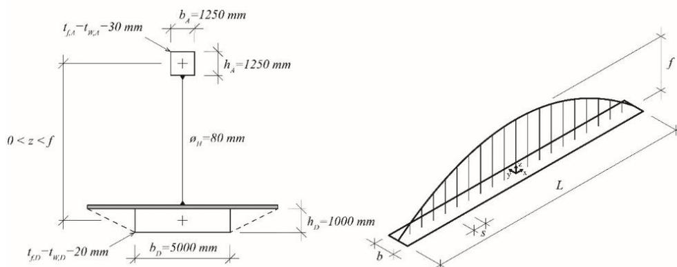
Fig. 12 Geometrical definition of the reference arch bridge (see Table 1)
