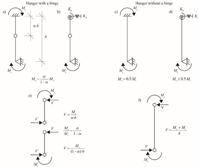
Fig. 24 Structural systems in hinged and non-hinged hangers
