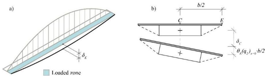
Fig. 18 (a) Deflected shape of the bridge under  $q_2$ . (b) deflected cross-section of the deck
