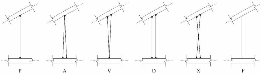
Fig. 29 Configurations of hangers within the plane of the arch
