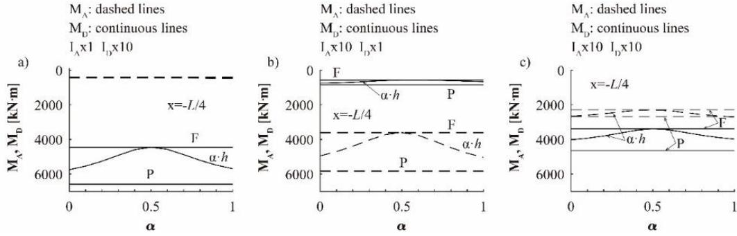
Fig. 17 Bending moment vs stiffness. In-plane stiffness of arch and deck factored, respectively, by  $k_A$  and  $k_D$ . (a)  $k_A = 1, k_D = 10$ ; (b)  $k_A = 10, k_D = 1$ ; (c)  $k_A = 10, k_D = 10$
