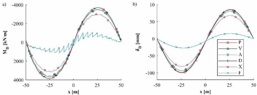
Fig. 31 Deck under  $q_3$ . (a) bending moments; (b) deflections at the centerline
