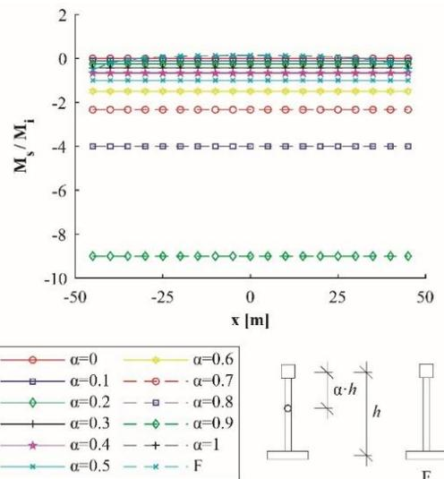
Fig. 25  $M_s/M_i$  for  $q_2$ . Reference model
