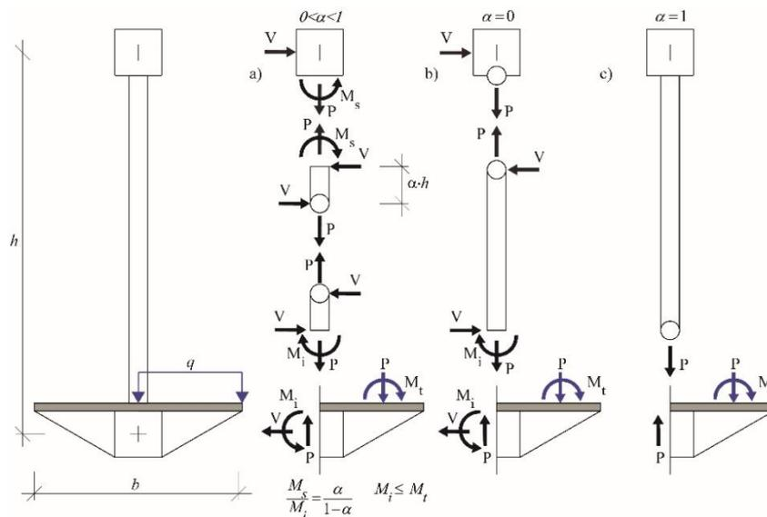
Fig. 22 Load transfer for asymmetrically loaded deck for the structural system composed of an arch and a hanger with a hinge
