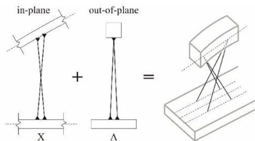
Fig. 33 Spatial cable arrangements obtained by combining most efficient planar configurations
