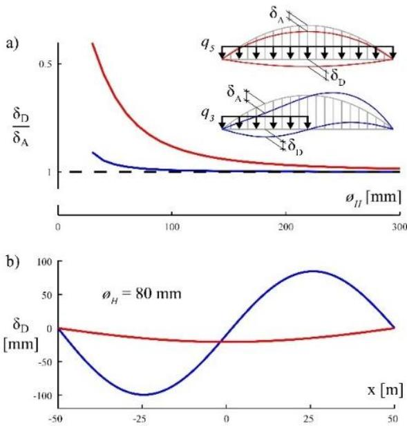
Fig. 14 (a) Ratio  $\delta_A/\delta_D$  vs. hanger diameter,  $\phi_H$ ; (b) Deck deflections  $\delta_D$  under  $q_3$  and  $q_5$  loads for  $\phi_H = 80$  mm
