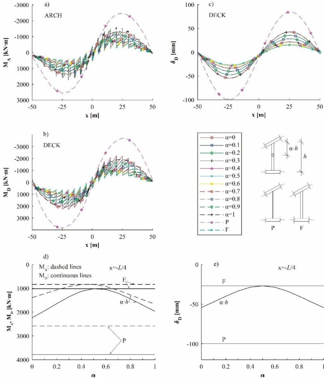
Fig. 16 (a) Arch and (b) deck bending moment diagrams vs. stiffness of hangers and hinge location; (c) Vertical deflection of the deck; (d) Bending moments detailed for quarter span; (e) Deck deflections detailed for quarter span
