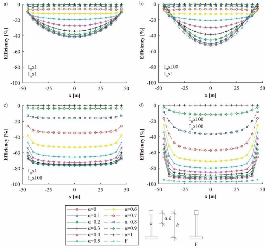
Fig. 23 Efficiency  $e_H = M_i/M_t$  vs stiffness. Transversal stiffness of hangers factored by  $k_H$ , and transversal and torsional stiffness of arch factored by  $k_A$ . (a)  $k_H = k_A = 1$ ; (b)  $k_H = 100, k_A = 1$ ; (c)  $k_H = 1, k_A = 100$ ; (d)  $k_H = k_A = 100$
