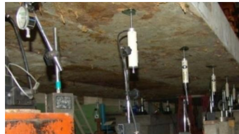
(c) Deployment of displacement sensors under the track slab
