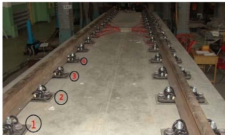
(b) Photography of the rail and fastener arrangement
