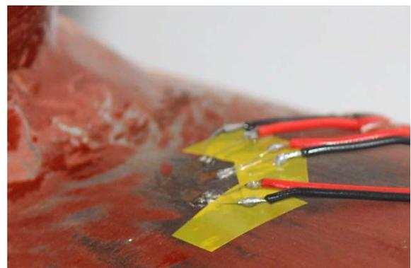
Fig. 5 Strain gauges fixed on the joint
