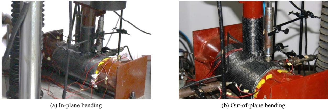
Fig. 17 Arrangement of CFRP wrapped T-joint specimen on UTM
