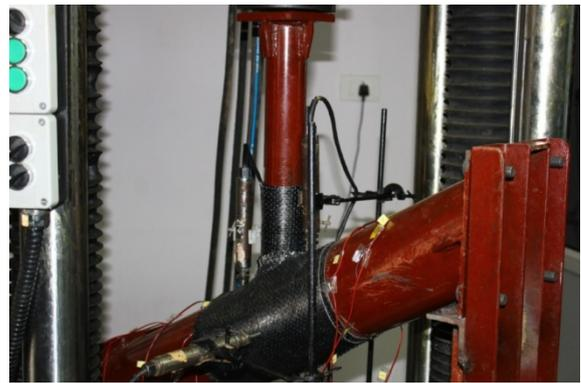
(b) CFRP strengthened Y-joint
