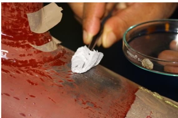
Fig. 4 Cleaning the location with acetone
