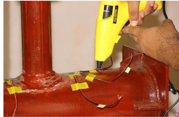
Fig. 7 Using hot glue fix the wires on to the joint
