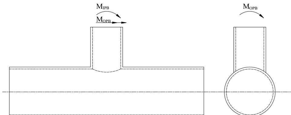
Fig. 12 In-plane bending moment and out-of-plane bending moment
