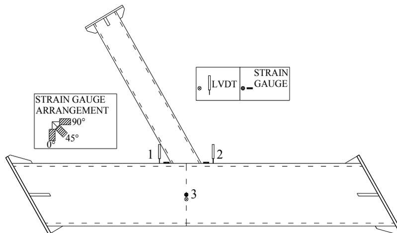
Fig. 3 Arrangement of LVDT and strain gauges for a Y-joint
