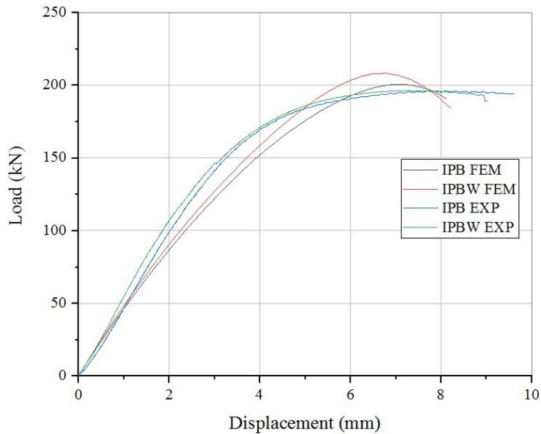
(IPB – Reference T-joint subjected to in plane bending; IPBW – CFRP strengthened T-joint subjected to in plane bending; FEM – finite element investigation; EXP – experimental technique)
