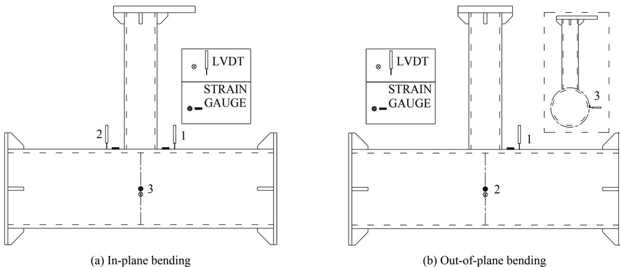
Fig. 14 Arrangement of LVDT and strain gauges for T-joint
