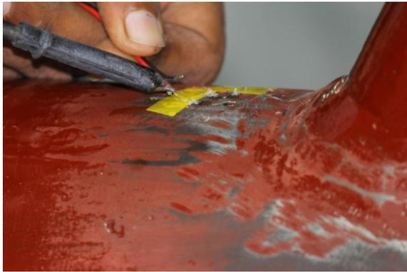
Fig. 6 Soldering the strain gauges to lead wires
