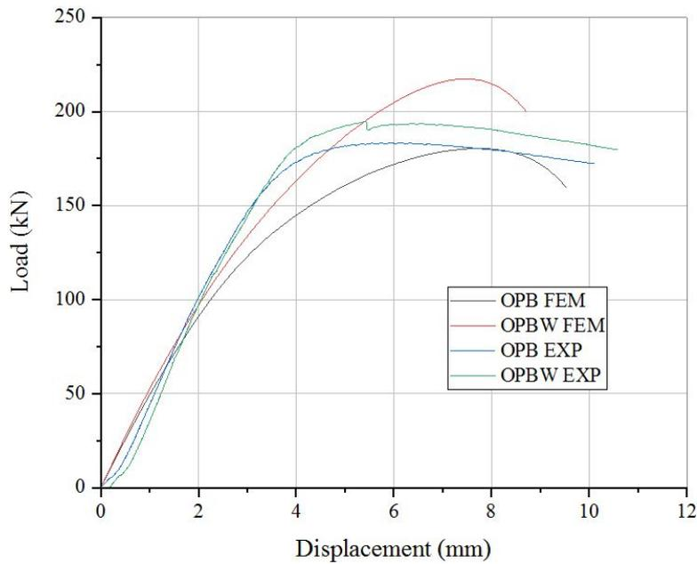
(OPB – Reference T-joint subjected to out of plane bending; OPBW – CFRP strengthened T-joint subjected to out of plane bending; FEM – finite element investigation; EXP – experimental technique)
