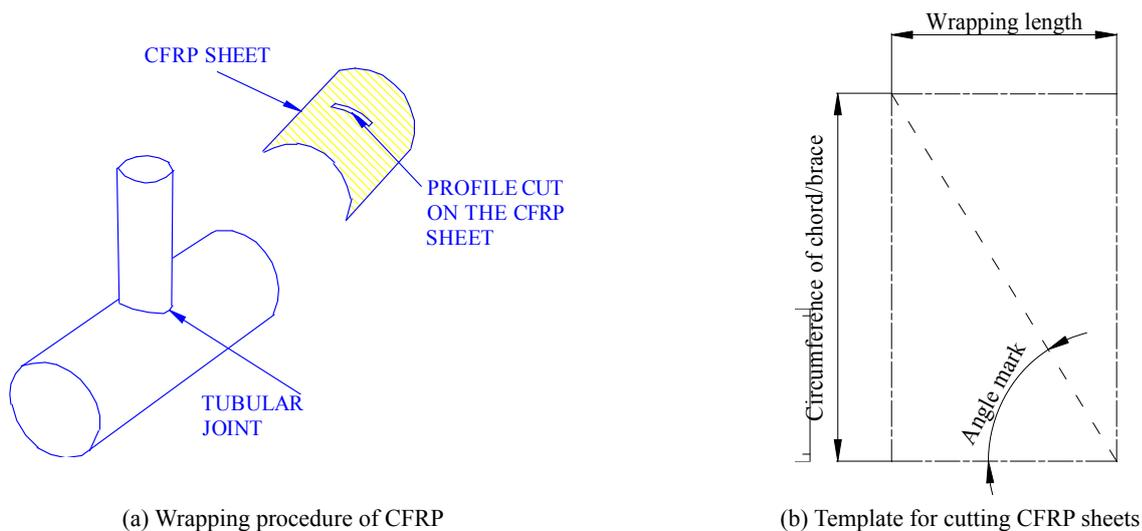
Fig. 15 Illustrating CFRP wrapping procedure on to the tubular joint
