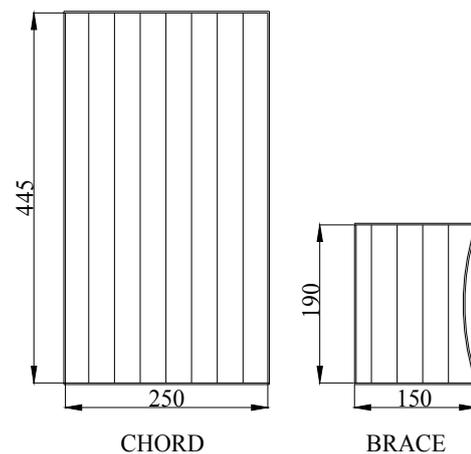
Fig. 9 Details of chord and brace template
