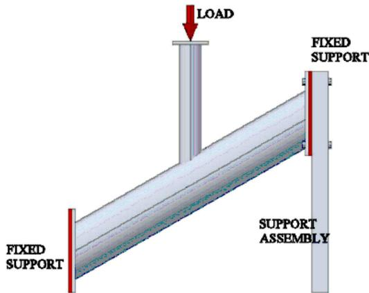
Fig. 2 General arrangement of Y-joint for axial loading
