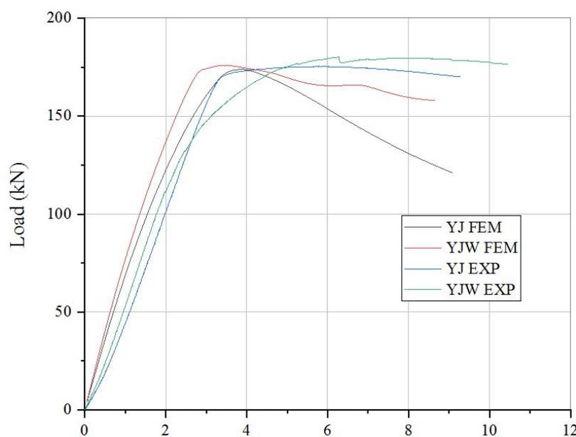
(YJ – Y-joint; YJW – CFRP strengthened Y-Joint; FEM – finite element investigation; EXP – experimental technique)
