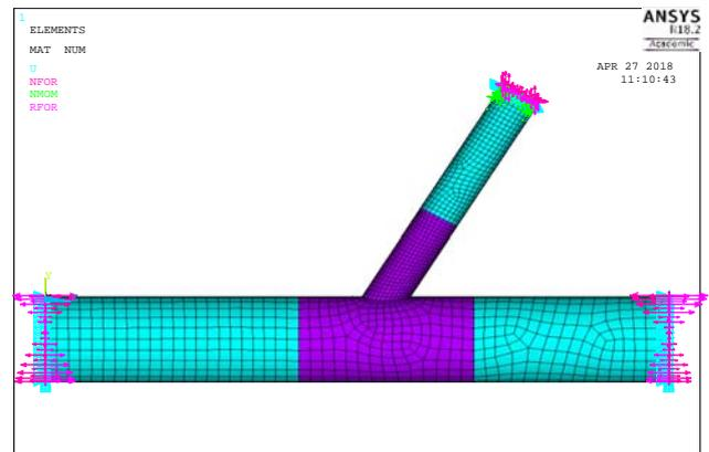
(b) CFRP strengthened Y-joint
