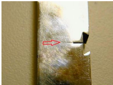
Fig. 5 Fatigue crack propagation
