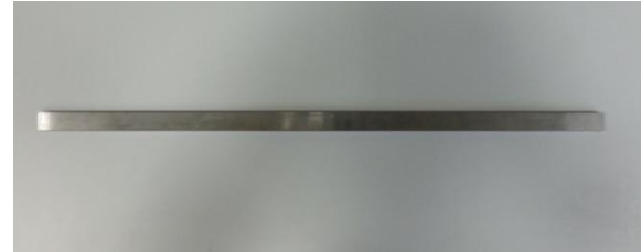
Fig. 1 8 \times 16 \times 500 mm beam produced from 4140 steel
