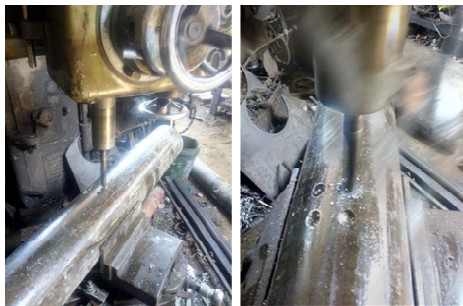
Fig. 2 Corrosion damage creation
