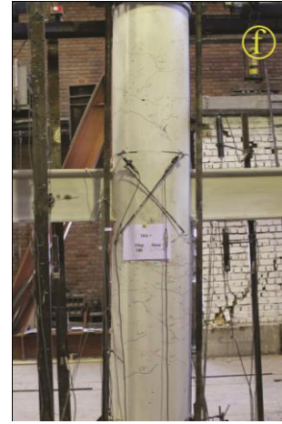
(f) Cracks on the column at about 6% storey drift
