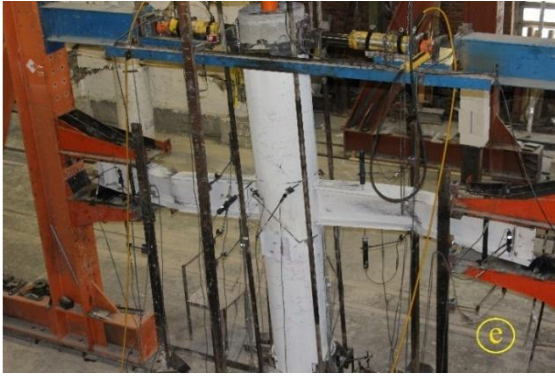
(e) Complete buckling of about 6% storey drift
