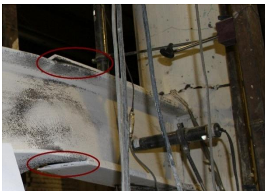
Fig. 6 Weld fracture on specimen 1 at 5% storey drift
