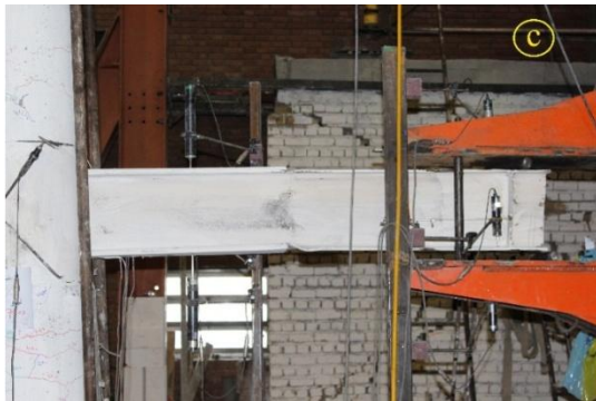
(c) Buckling of beam flange at about 5% storey drift
