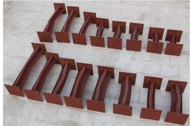
Fig. 8 Photograph of the back-to-back built-up CFS angle sections at failure from experiments
