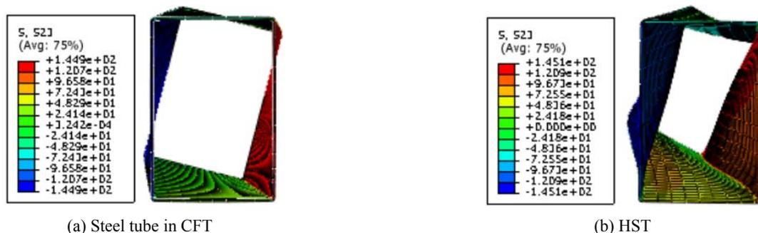
Fig. 4 Typical failure modes of steel tube in CFT column and HST
