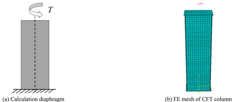
Fig. 1 Established FE model of rectangular CFT columns under pure torsion
