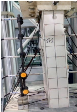
(a) Deformation of the specimen at failure
