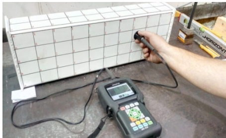
(b) Measurement of the width of walls in the short specimens
