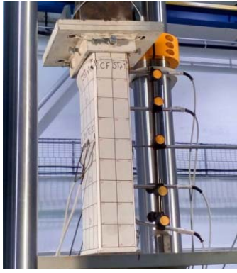
(a) Deformation of the specimen at failure
