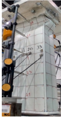
(a) Deformation of the specimen at failure
