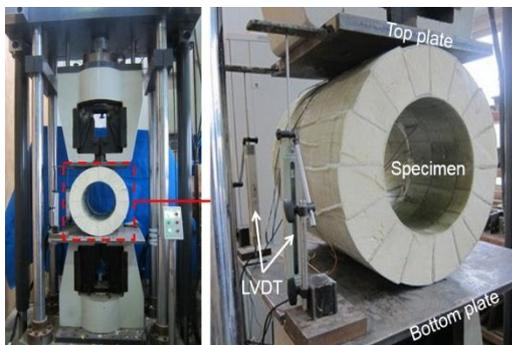
(a) Loading test set-up for specimen
