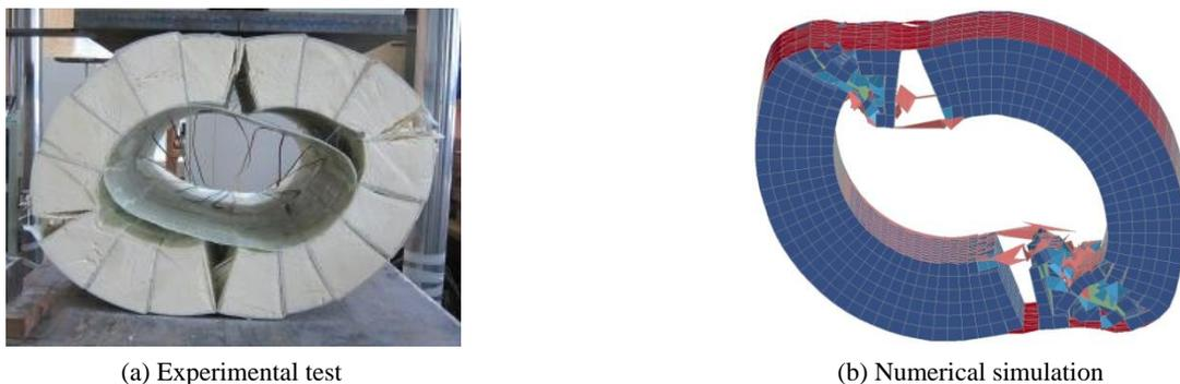
Fig. 20 Crushed shape of specimen D500-L16-T5
