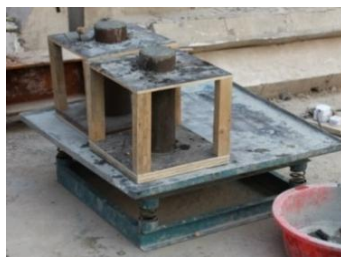
(a) The wooden mold
