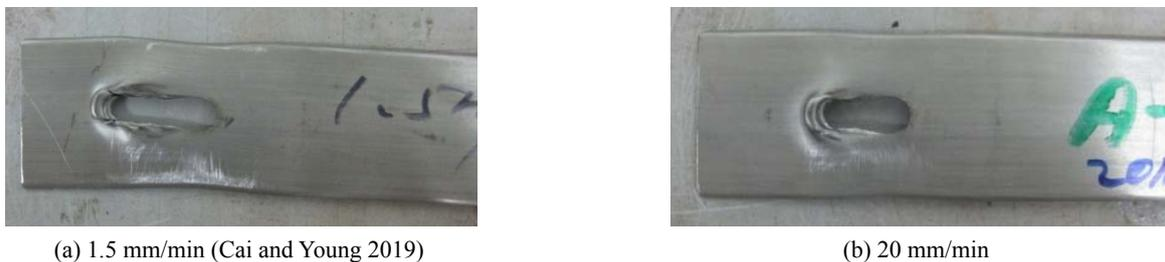
Fig. 17 Bearing failure mode of specimen Series D-A-1-10 under different strain rates
