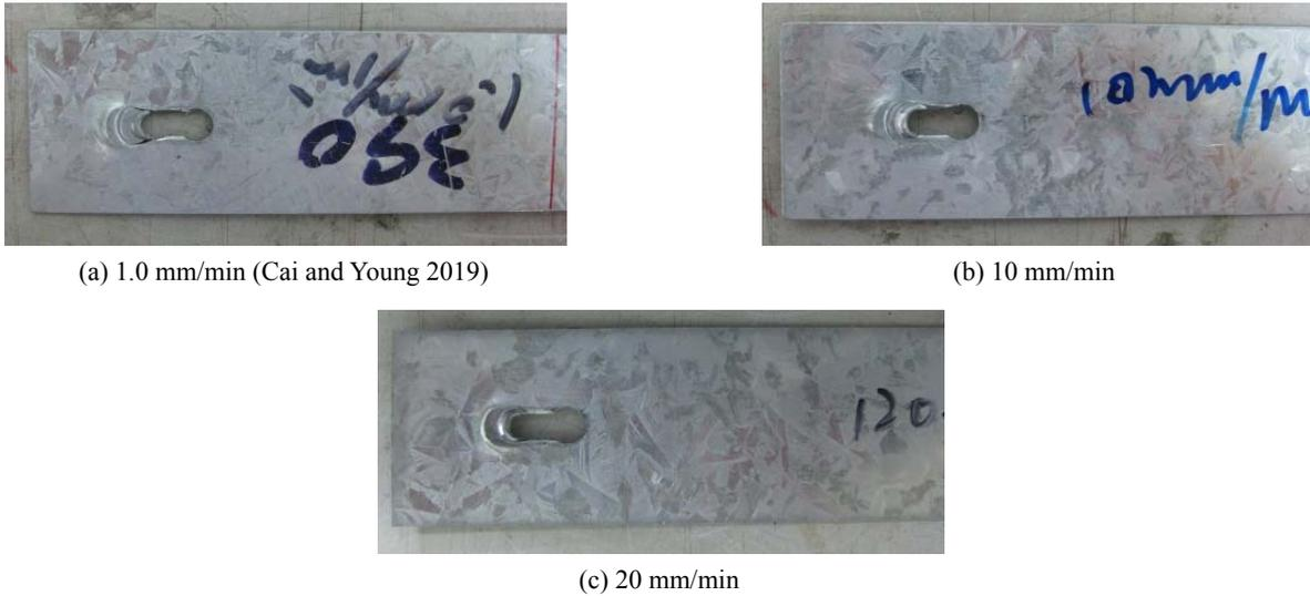
Fig. 15 Bearing failure of specimen Series D-120-1-8 under different strain rates
