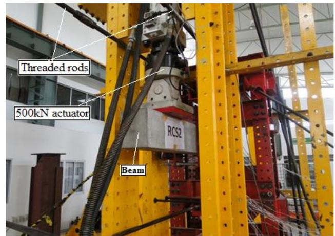
Fig. 9 Position of 500 kN actuator
