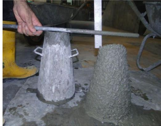
Fig. 5 Concrete specimen casting and concrete slump measurement
