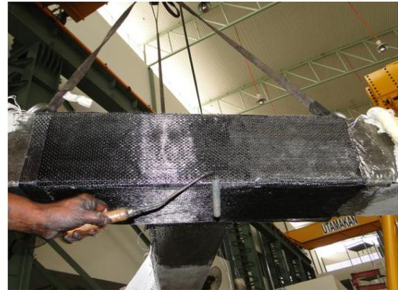
Fig. 8 Installation of CFRP plate on specimen RCS5 and CFRP wrapping of specimen RCS6
