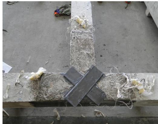
Fig. 6 Concrete cylinders for testing the material properties and Installation of CFRP plate on specimen RCS2
