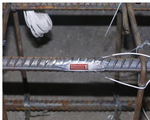
Fig. 4 Concrete specimen casting and strain gauge installation
