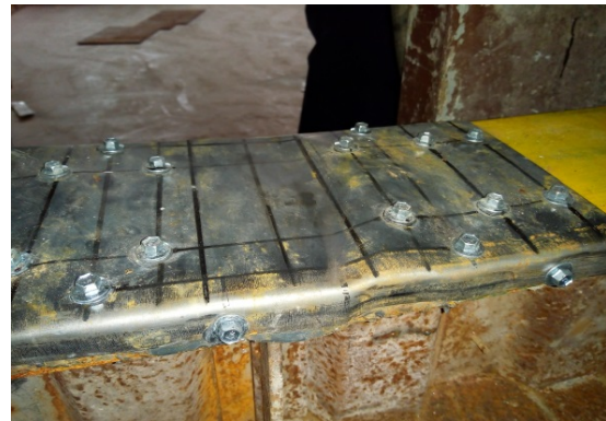
(b) Local flange buckling in Model A2
