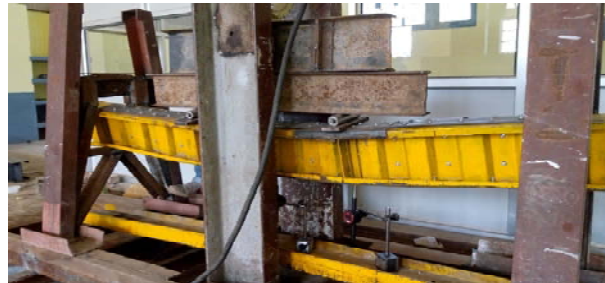
(c) Lateral torsional buckling
