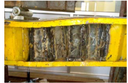
(c) Local flange buckling
