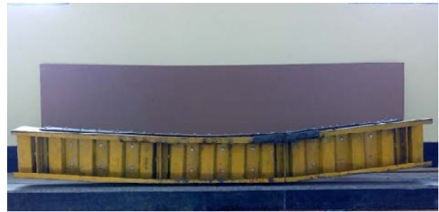
(b) Failure in Model A4
