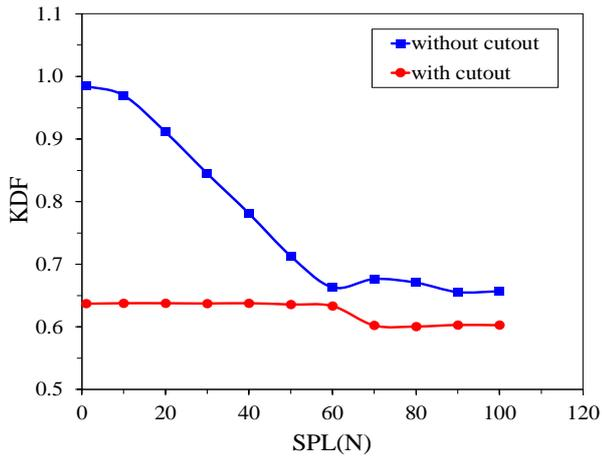
Fig. 6 Effect of cutout on KDF of a composite cylindrical shell
