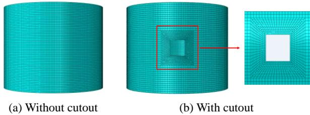
Fig. 3 Mesh density in finite element model of composite cylinders
