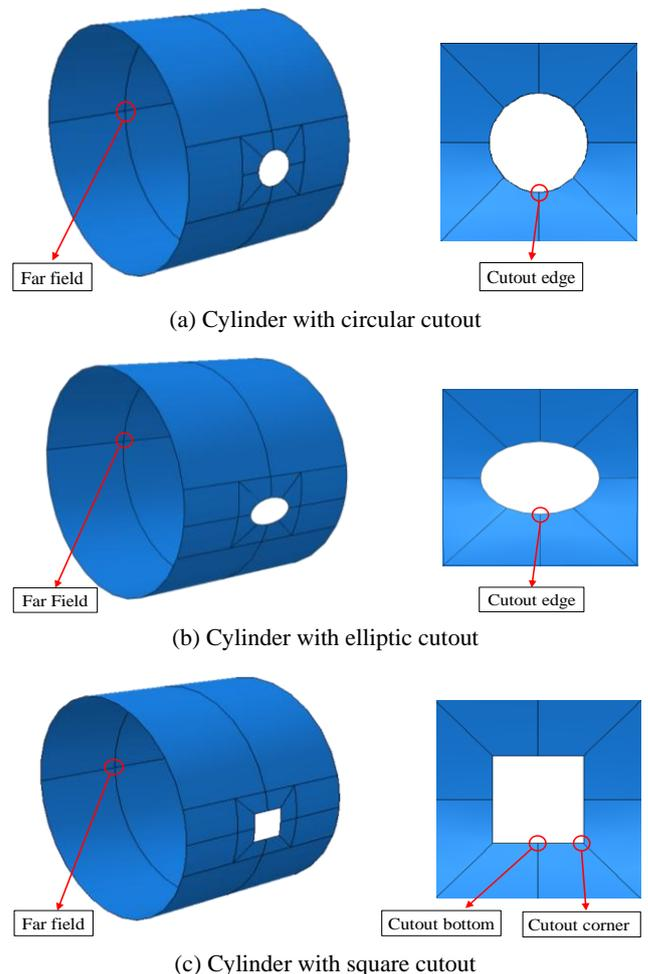
Fig. 10 Locations of single perturbation load in cylinders with cutout
