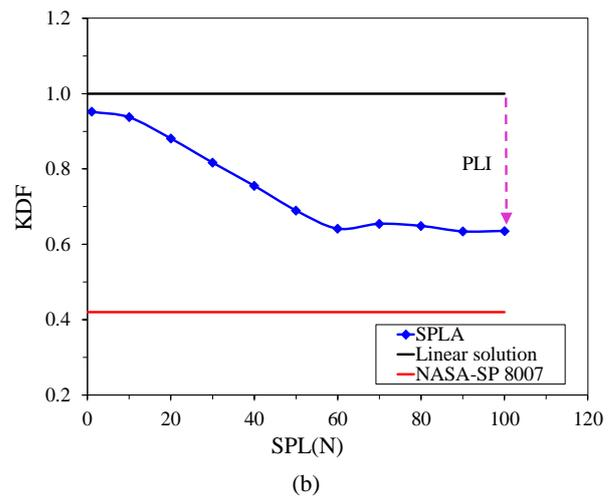
Fig. 7 Effect of increasing single perturbation load on load-end shortening and KDF of carbon/epoxy cylindrical shell
