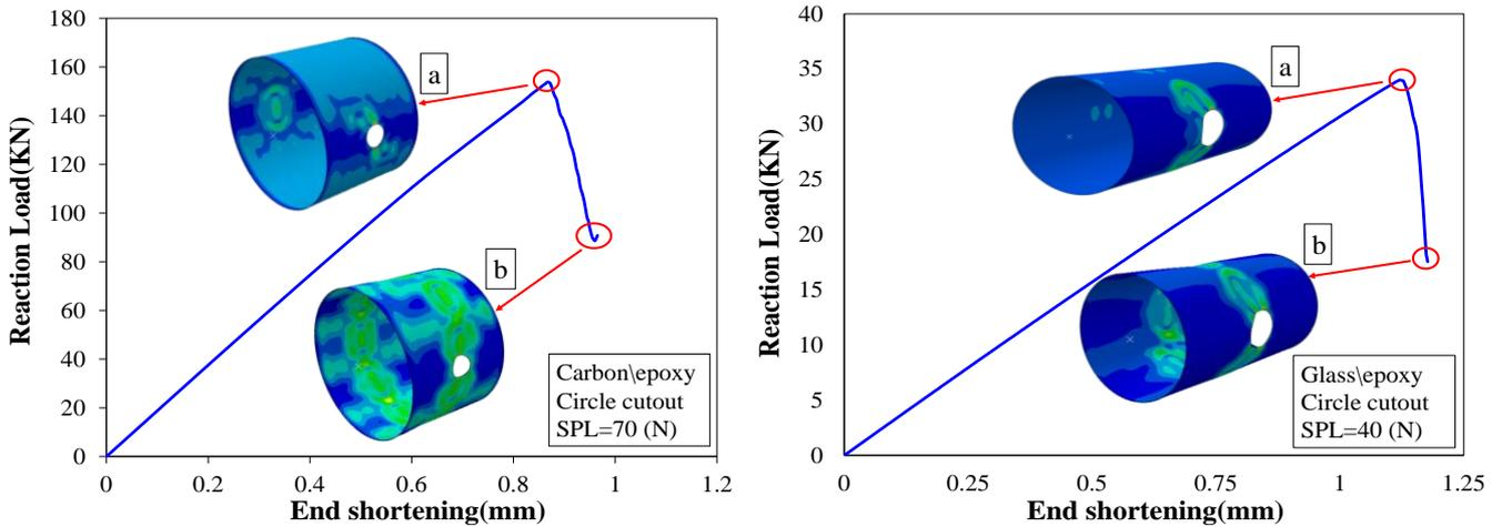
Fig. 9 Load-end shortening curves from nonlinear analysis with SPLA
