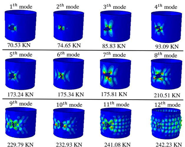
Fig. 5 Twelve mode shapes of carbon/epoxy cylindrical shell with circular cutout using linear buckling analysis
