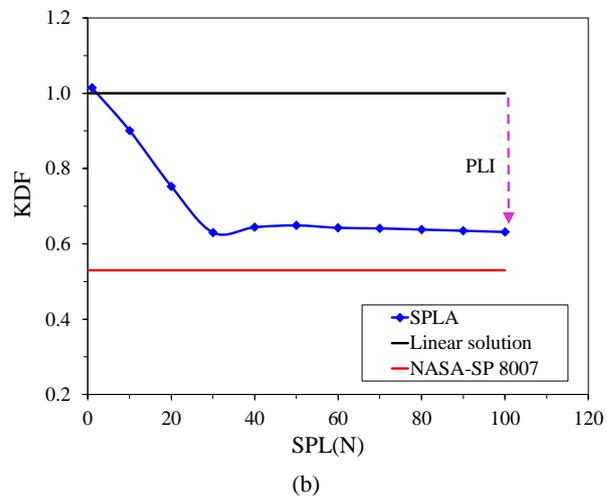
Fig. 8 Effect of increasing single perturbation load on the load-end shortening and KDF of glass/epoxy cylindrical shell
