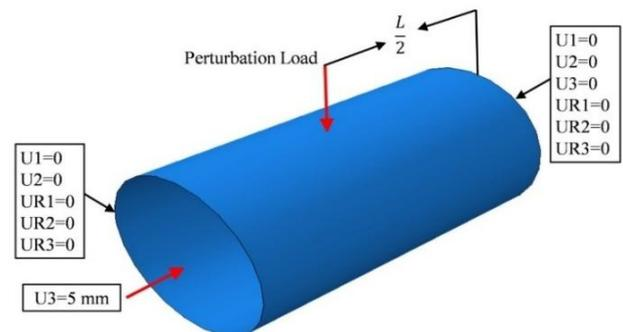
Fig. 2 Boundary conditions and location of applying single perturbation load
