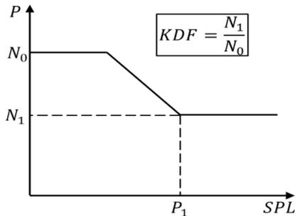
Fig. 4 Variation of buckling load according to SPL
