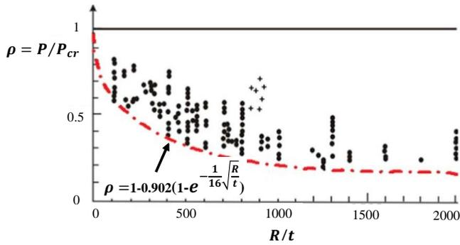
Fig. 1 Experimental data for an isotropic cylindrical shell under axial compressive load (modified by Arbocz and Starnes 2002)
