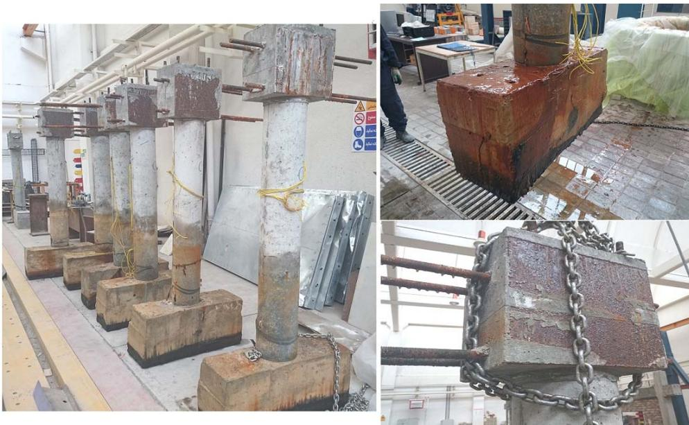
Fig. 4 The condition of damages in columns components after corrosion process
