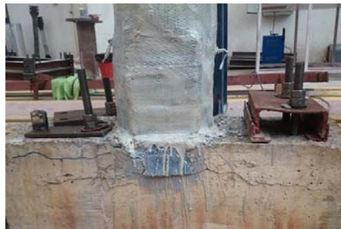
(g) Specimen C7-TP-2CF at failure
