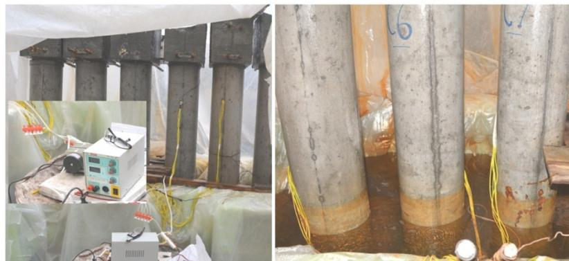
Fig. 3 A perspective of accelerated corrosion setup
