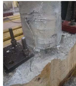
(f) Specimen C6-CF-BP-CF at failure
