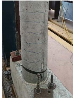
(b) Specimen BEN2 at failure
