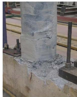
(e) Specimen C5-BP-2CF at failure
