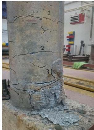
(a) Specimen BEN1 at failure
