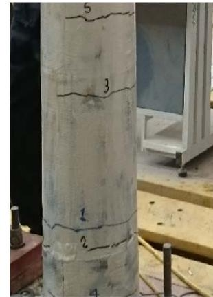
(c) Specimen C3-2CF at failure
