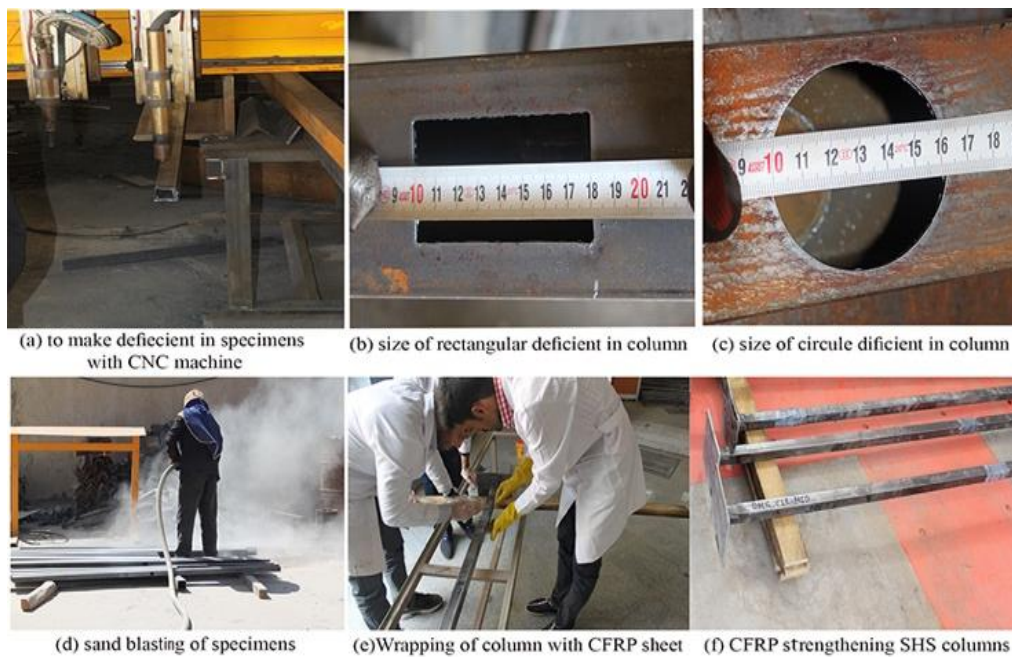
Fig. 5 Preparation of CFRP-strengthened specimens
