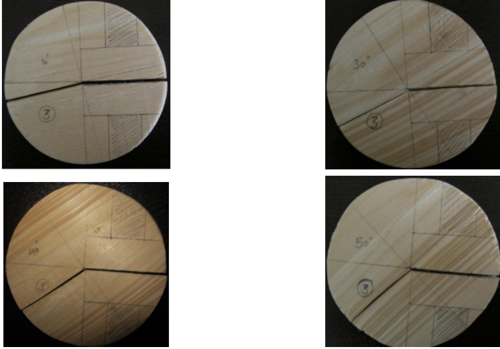
Fig. 1 Propagation of cracks along fiber direction and in isotropic medium between fibers (Farid and Fakoor 2019)
