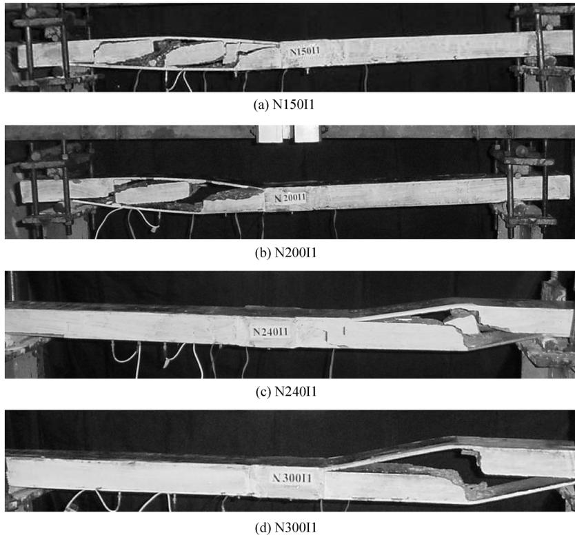
Fig. 4 Failure pattern of beams under impact loading with drop height 1 meter; (a) N150I1 (b) N200I1 (c) N240I1 (d) N300I1
