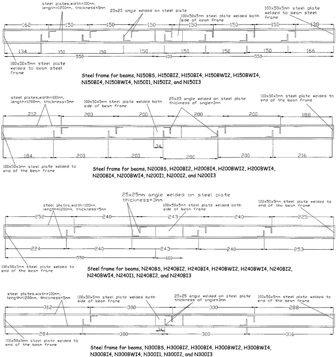
Fig. 1 Details sandwich beam specimen
