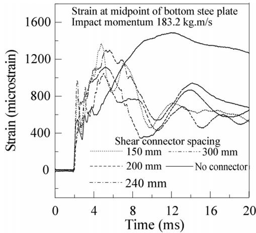
Fig. 16 Effect of shear connector spacing; strain time history (projectile mass 43 kg)
