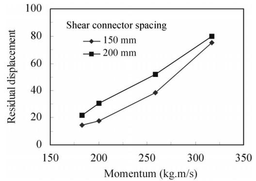
Fig. 9 Effect of momentum on residual displacement of sandwich beams (projectile mass 43 kg)
