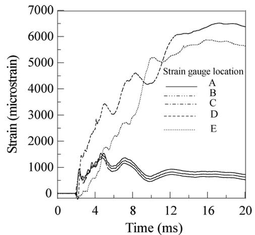
Fig. 15 Strain time response of bottom steel plate of beam N150I1 under impact momentum 183.2 kg.m/s
