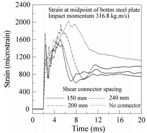
Fig. 17 Effect of shear connector spacing; strain time history (projectile mass 43 kg)
