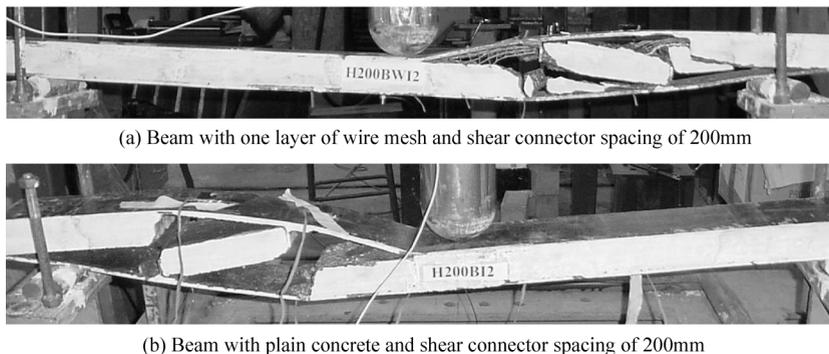
Fig. 7 Comparing the damage between beams with wire mesh and without wire mesh
