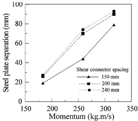
Fig. 8 Effect of impact momentum on steel plate separation (projectile mass 43 kg)
