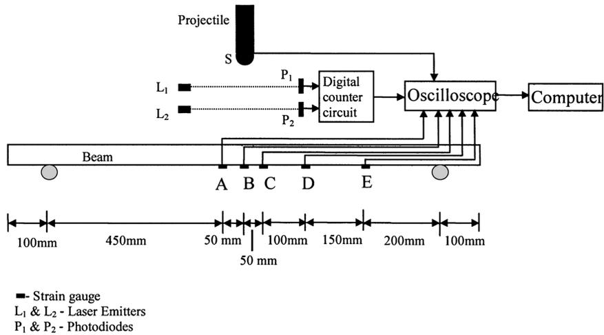
Fig. 3 Schematic diagram of instrumentation and data acquisition system
