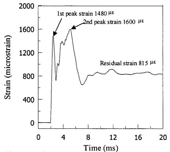
Fig. 13 Strain response of bottom steel plate at midpoint of sandwich specimen N150I3 with impact momentum 316.8 kg.m/s
