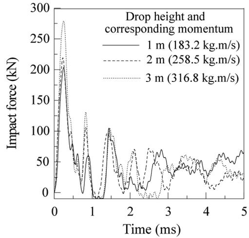
Fig. 11 Impact force time history of beams with different drop height (connector spacing 150 mm)
