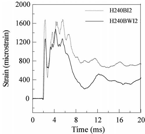
Fig. 18 Effect of wire mesh on strain at mid point of bottom steel plate upon impact (impact momentum 200.7 kg.m/s)
