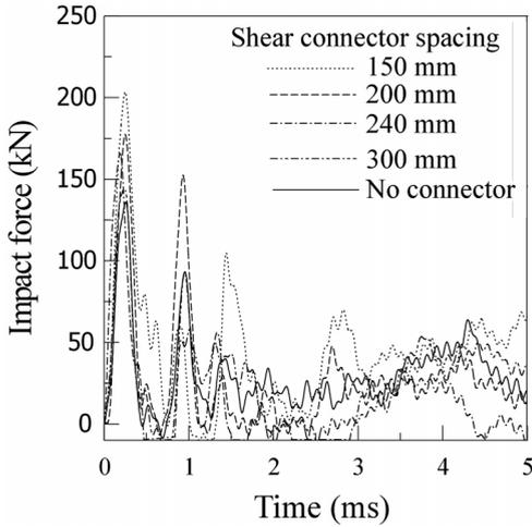
Fig. 10 Effect of shear connector spacing (impact momentum 183.2 kg.m/s)
