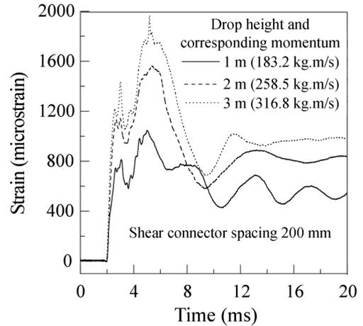
Fig. 19 Strain-time history of beams with different drop height (projectile mass 43 kg)
