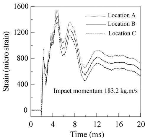
Fig. 14 Strain response of sandwich specimens N150I1 under impact
