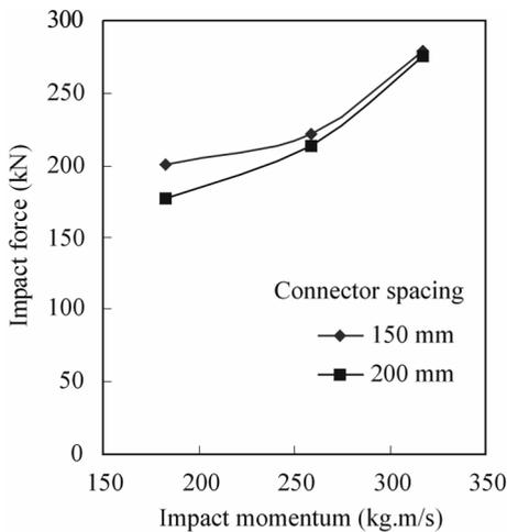
Fig. 12 Effect of impact momentum on impact force of sandwich beams.
