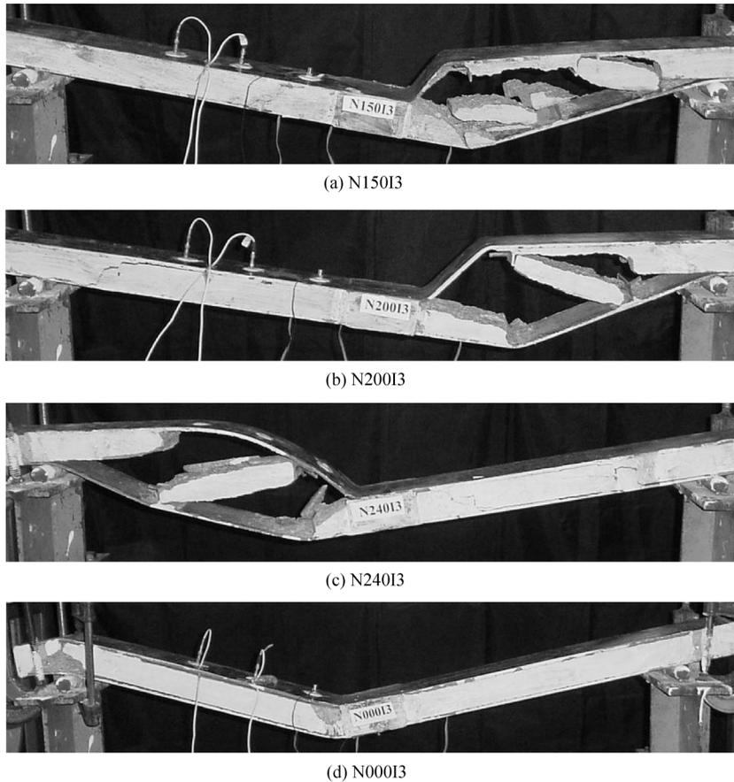
Fig 6 Failure pattern of beams under impact load with drop height 3 meter; (a) N150I3 (b) N200I3 (c) N240I3 (d) N000I3.
