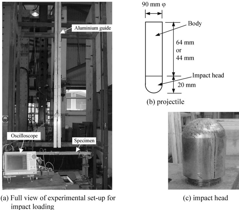
Fig. 2 (a) Full view of experimental set-up for impact loading (b) projectile and (c) impact head
