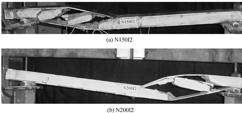
Fig. 5 Failure pattern of beams under impact loading with drop height 2 meter; (a) N150I2 (b) N200I2
