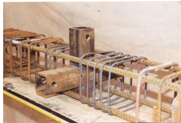
Fig. 7 Column reinforcement with RHS billet
