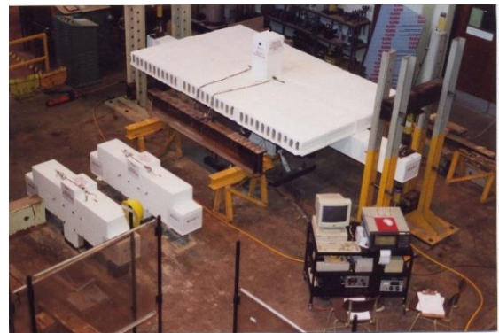
Fig. 15 Test arrangements to study semi-rigid internal beam-to-column connections
