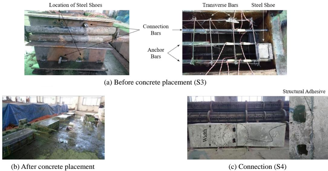
Fig. 3 Production and connection of test specimens
