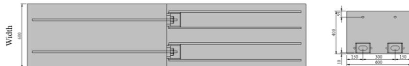
(d) Top view and section of S4: 2 Pairs of connectors (Bisymmetric)
