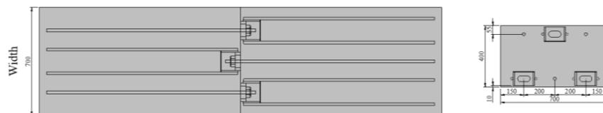
(e) Top view and section of S5: 3 Pairs of connectors
