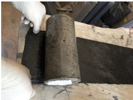
(c) Application and impregnation of the FRP fabric
