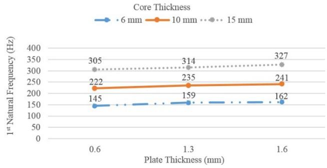
(b) PU foam filled honeycomb sandwich structures
