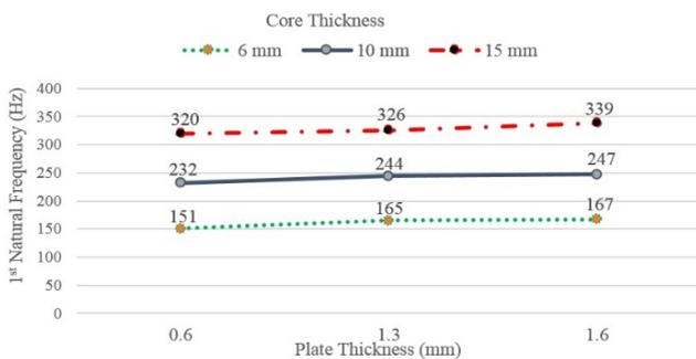
(a) Hollow honeycomb sandwich structures
