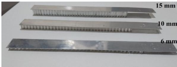
Fig. 2 Honeycomb sandwich specimens having different core thicknesses formed for use in experimental studies
