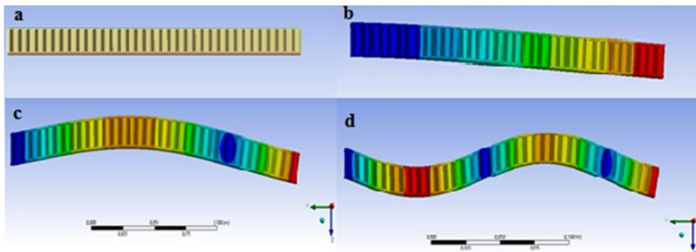
Fig. 7 The model and first three mod shapes
