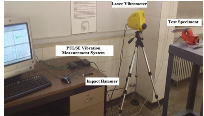
Fig. 3 Experimental system used to determine vibration characteristics
