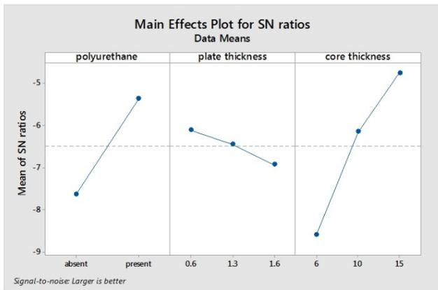
Fig. 13 Plots of main parameters affecting the damping ratio according to the S / N ratios
