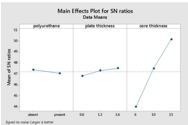
Fig. 12 Plotting the main parameters affecting the 1<sup>st</sup> natural frequency according to the S/N ratios
