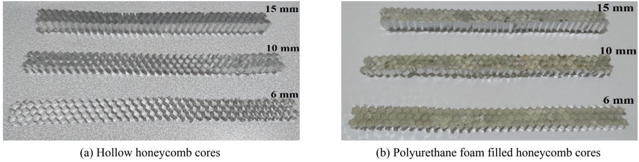
Fig. 1 Hollow and foam filled aluminum honeycomb cores at different thicknesses used in the production of sandwich structures
