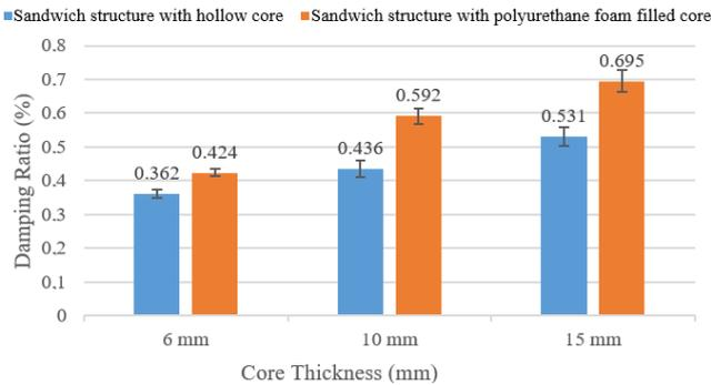
Fig. 11 Influence on damping ratio of hollow and polyurethane foam filled cores and core thickness (for 0.6 mm face sheet thickness)
