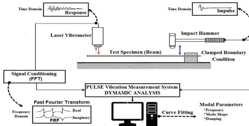
Fig. 4 Schematic representation of the experimental vibration measurement system
