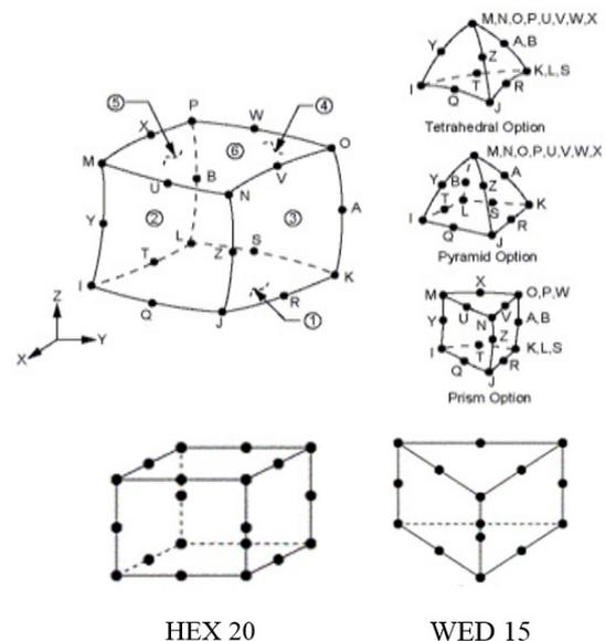
Fig. 5 Element types used in meshing
