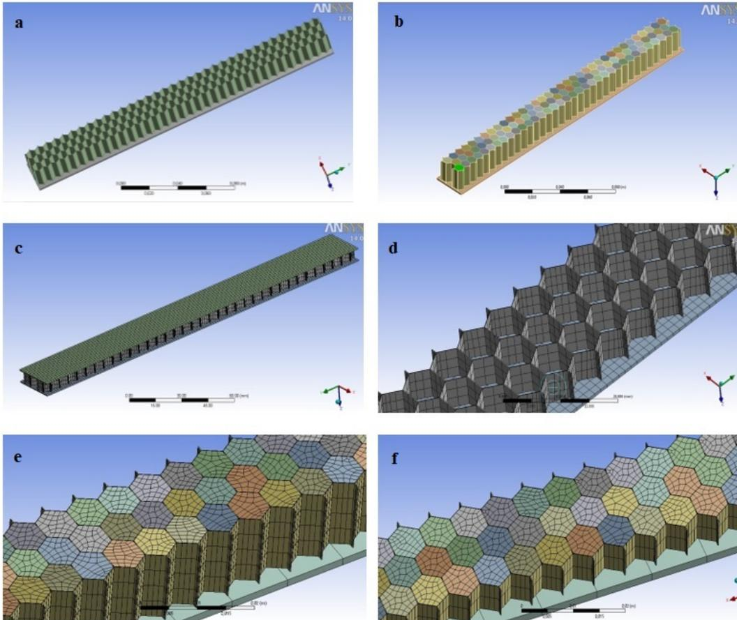
Fig. 6 Sandwich structures that filled with PU foam and hollow, and mesh samples used in numerical analysis
