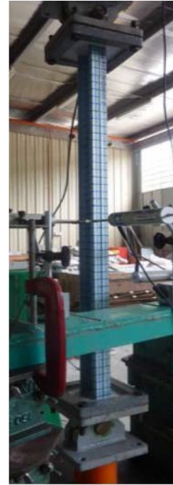
Fig. 4 Photograph of test set-up for back-to-back built-up CFS un-lipped-channel sections (Ting et al. 2018)
