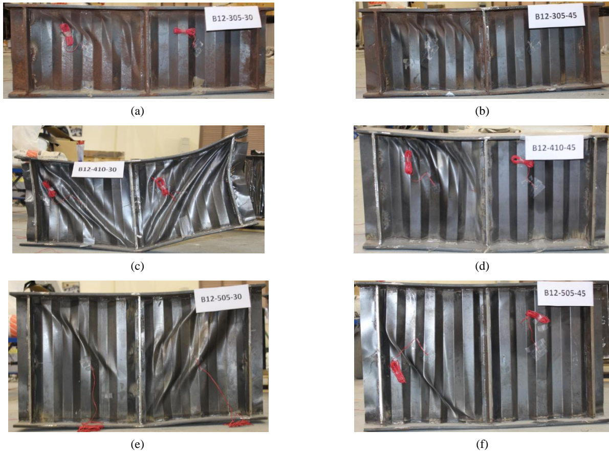
Fig. 17 Failure modes of tested beam specimens
