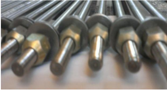
Fig. 5 Mechanical anchorage of SMA bars
