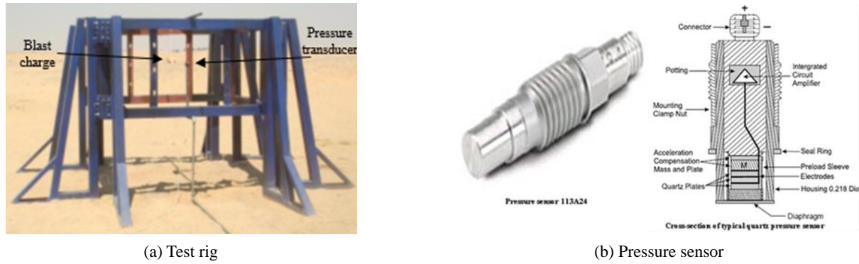
Fig. 2 Structural steel frame for explosion field tests and sensor reading of 1 kg TNT at 1 m
