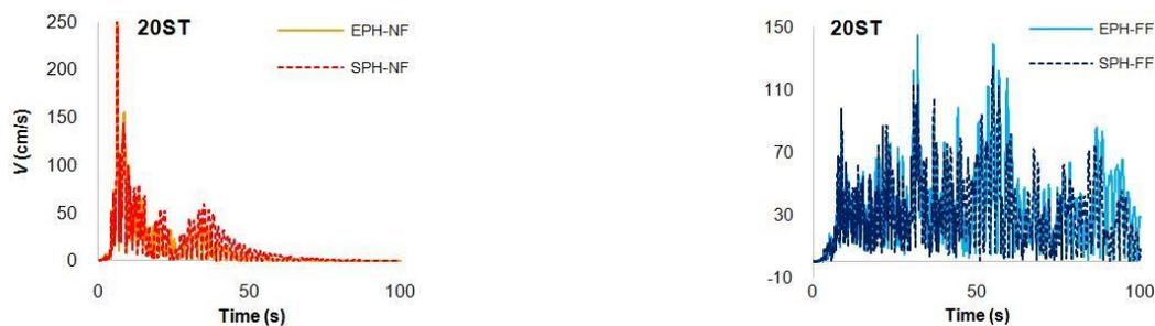
Fig. 12 Kinetic energy pertaining to the 20-storey-SPH and -EPH subjected to sample the NF and FF earthquakes
