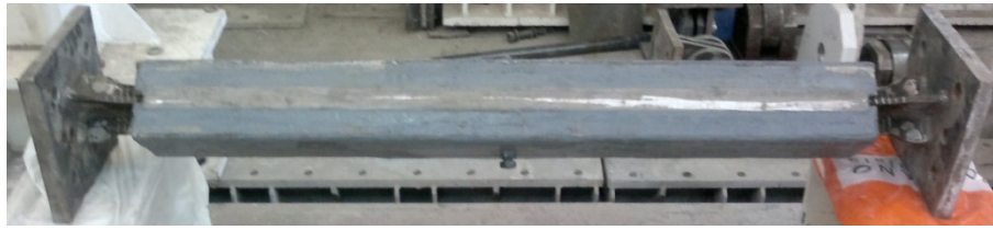
(d) Assembled BRB after covering concrete blocks with resin-based primer
