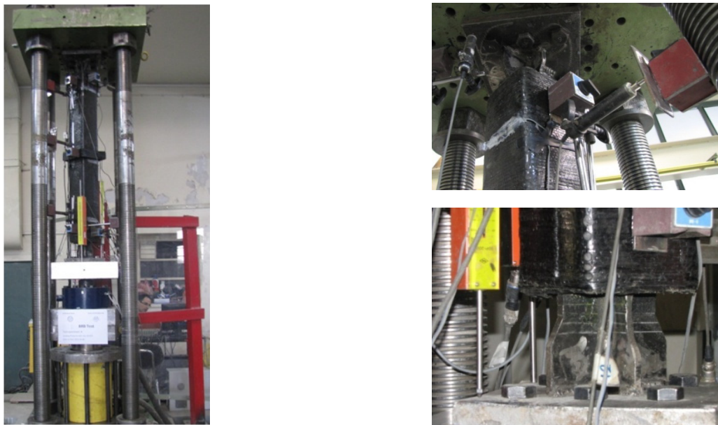
Fig. 23 Specimen 2 in the uniaxial test setup
