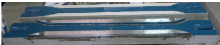
(b) Painting ceramic paste on the inner surface of encasing
