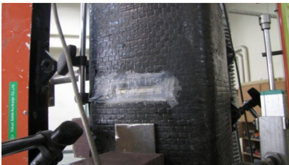
Fig. 15 Sample strain gauge on encasing
