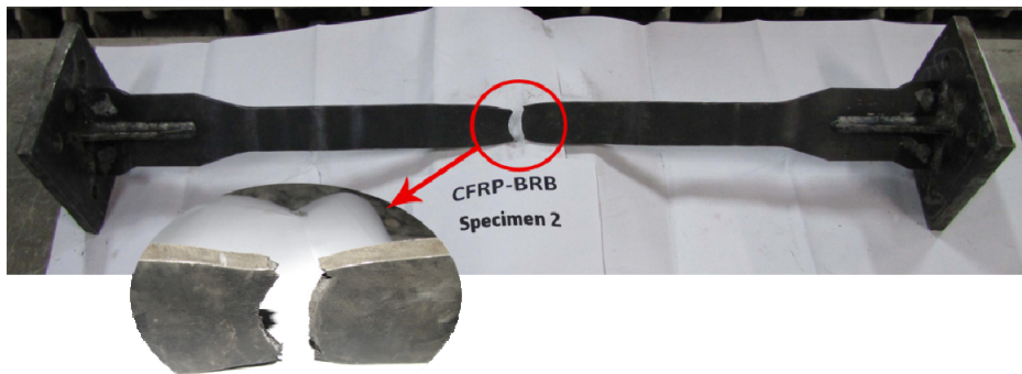
Fig. 25 Core of specimen 2 after test
