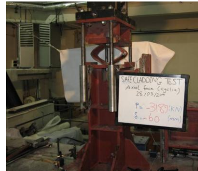
(a) Axial (transversal) loading (Position A)
