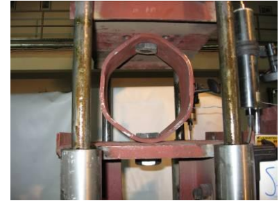
(c) Deformed shape for tension
