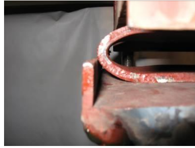
(b) Deformed shape for compression
