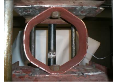
(c) Deformed shape for tension
