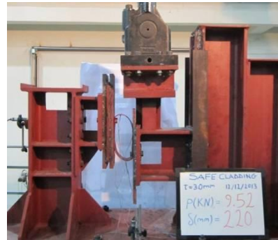
(b) Shear (longitudinal) loading (Position B)
