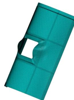
Fig. 13 Mesh with the geometric imperfection amplified with a factor of 200
