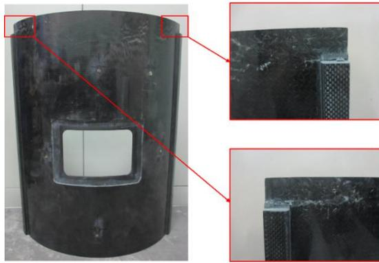
Fig. 7 Cracks close to upper end of the specimen
