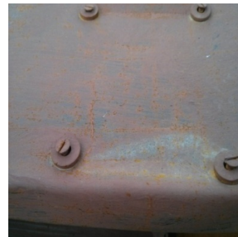
(b) Compression flange buckling in Model A
