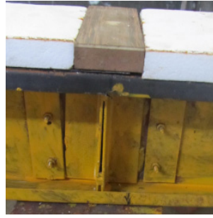
(b) Wooden bearing under loading points in Model C
