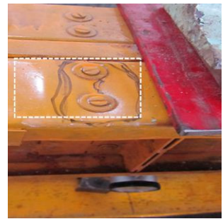
(c) Flange buckling in Model D
