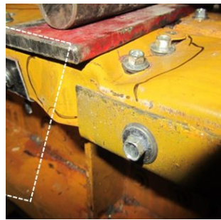
(b) Flange buckling in Model F
