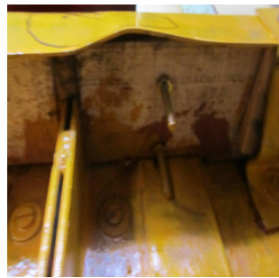
(b) Lip buckling in Model D
