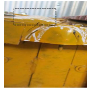
(c) Flange buckling in Model E
