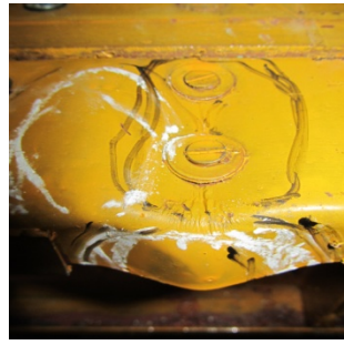
(b) Lip buckling in Model E
