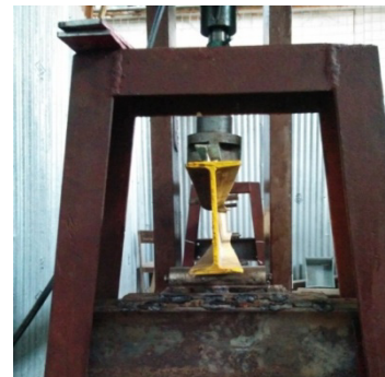
(b) Lateral buckling mode in Model G
